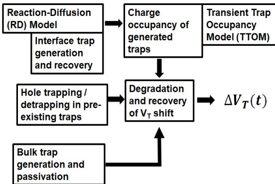
Fig. 5. Schematic of a BAT (BTI Analysis Tool) framework consisting of uncorrelated  $\Delta V_{IT}$ ,  $\Delta V_{HT}$  and  $\Delta V_{OT}$  components.
