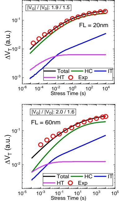
Fig. 16. Overall  $\Delta V_T$  under  $V_G > V_D$  stress for  $FL$  of 20nm (top) and 60nm (bottom).  $\Delta V_{IT}$  kinetics is simulated using TCAD for NBTI with SH. Symbols: Exp Data; Lines: Simulation
