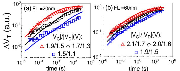
Fig. 17. Time kinetics of measured and modeled  $\Delta V_T$  at different stress  $V_G/V_D$  conditions, for (a)  $FL = 20 \text{ nm}$  and (b)  $FL = 60 \text{ nm}$  devices. Symbols: data, lines: model.
