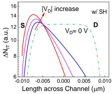
Fig. 12. Spatial distribution of effective  $\Delta N_{IT}$  across the channel with varying  $V_D$  with SH. Source (S) and Drain (D) side are marked.
