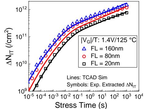
Fig. 8. TCAD modeling of BAT extracted  $\Delta N_{IT}$  stress time kinetics for different FL for fixed  $V_G$  and  $T$  conditions.
