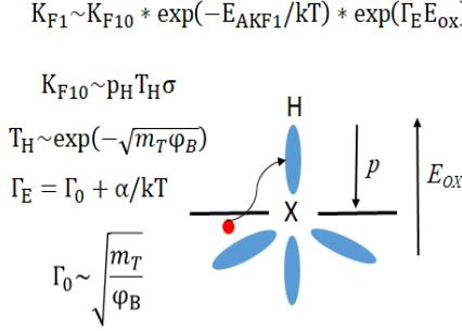
Fig. 3. Schematic of Si-H bond dissociation at the channel/IL interface. Inversion layer holes tunnel into interfacial Si-H bonds aided by the oxide electric field ( $E_{ox}$ ).
