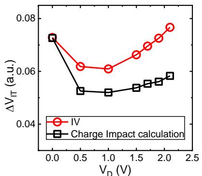
Fig. 14.  $\Delta V_T$  using avg.  $N_{IT}$  and transfer IV under NBTI stress as a function of  $V_D$ . Note that charge impact calculations are not valid due to localized trap generation under non-zero  $V_D$ . Post stress IV is needed for degradation calculations.
