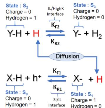
Fig. 2 MSC-HCD TCAD framework for interface trap generation.  $k_{FI}$  is bond dissociation rate and comes from CED model. Details in [7].
