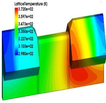
Fig. 11. 3D Lattice Temperature Profile along the channel in presence of  $V_D$ . Due to SH localized temperature rise at the drain side.
