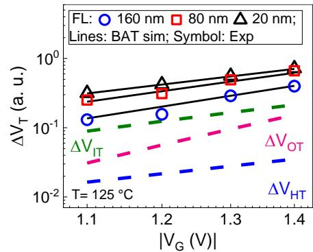
Fig. 7. Modeling of measured fixed time  $\Delta V_T$  as a function of  $V_G$  for a fixed  $T$  for different FL. Sub-components of overall  $\Delta V_T$  for FL 20 nm is shown.
