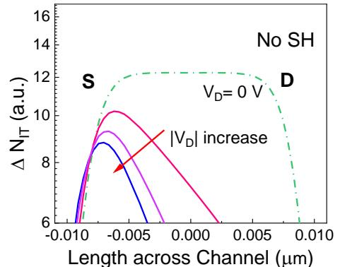
Fig. 10. Spatial distribution of  $\Delta N_{IT}$  across the channel with varying  $V_D$  without SH. It shows the reduction of  $\Delta N_{IT}$  due to decrease in vertical field (responsible for BTI) as  $V_D$  increase. Source (S) and Drain (D) side are marked.
