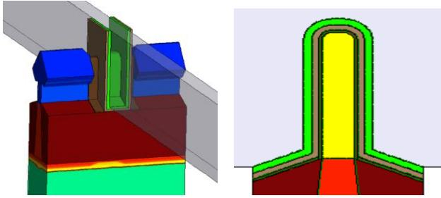
Fig. 4 (a) Isometric view of a 3D p-FinFET structure (FL = 20nm,) having raised epitaxial SiGe S-D and lateral Tungsten backend for H<sub>2</sub> diffusion. (b) 2D cross section of the fin showing IL, High-K, TiN cap and Tungsten layers in the gate stack
