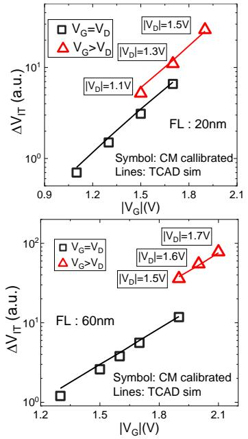
Fig. 15. Fixed time  $\Delta V_{IT}$  simulated using TCAD under different stress bias ( $V_G$  and  $V_D$ ) for  $FL$  of 20nm (top) and 60nm (bottom).
