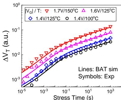
Fig. 6. Time evolution of ultrafast (10μs) measured  $\Delta V_T$  for DC stress with model estimation at multiple  $V_G$  and  $T$  for FL 20nm.
