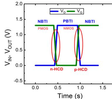
Fig.1. Time dependence of  $V_G$  and  $V_D$  and degradation mechanism in RO.
