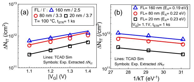
Fig. 9. (a) Fixed time  $\Delta N_{IT}$  as a function of  $V_G$  is shown for a fixed  $T$ , (b) plots fixed time  $\Delta N_{IT}$  as a function of  $T$  for a fixed  $V_G$  for different FL. Symbol: BAT extracted; Lines: TCAD
