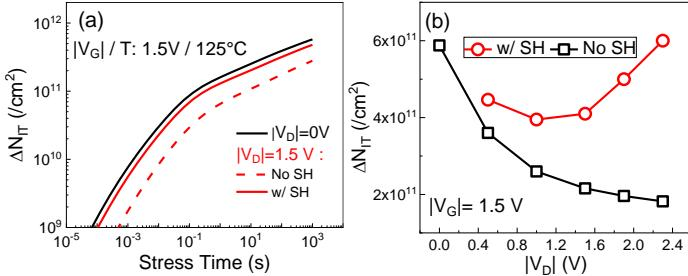
Fig. 13. (a) TCAD extracted  $\Delta N_{IT}$  time kinetics for different  $V_D$  and (b) fixed time  $\Delta N_{IT}$  as a function of  $V_D$ , with and without SH, at fix  $V_G$ .
