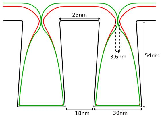
Fig. 5: Slice of a three-dimensional emulation of the pinch-off plasma CVD process inside tapered trenches (black surface). The green surface is the result of the geometric advection, while even the most robust iterative scheme (SLLF [11], red surface) is unable to predict the closing of the trench.
