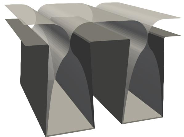
Fig. 4: Result of three-dimensional emulation of the pinch-off plasma CVD model. As expected, the resulting surface is pinched off exactly since the advection is purely geometric.
