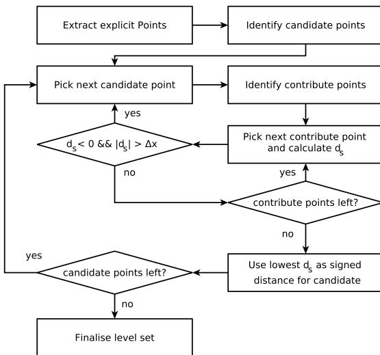
Fig. 2: Flowchart of the geometric advection algorithm.
