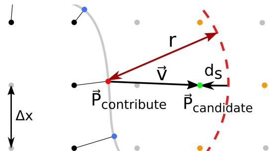
Fig. 1: Signed distance calculation for candidate point  $\vec{P}_{candidate}$  (green) from an explicit point  $\vec{P}_{contribute}$  (red) on the initial surface. The spherical distribution is depicted by the dashed red circle.  $d_s$  is then used as the new LS value for the grid point  $\vec{P}_{candidate}$ . The LS grid spacing is shown as  $\Delta x$ .
