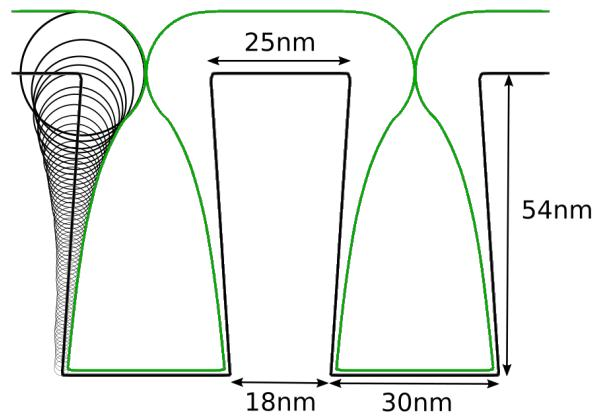
Fig. 3: Schematic showing how the described model creates the resulting geometry (green) using spherical geometric distributions (black circles). The outline of the circles thus creates the final geometry, based on the view factor calculated using Eq. (3).
