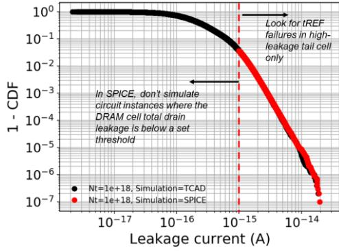
Figure 8: CCDF of leakage current in the DRAM cell: TCAD vs SPICE simulation. The SPICE tail methodology allows fast and reliable high-sigma analysis.
