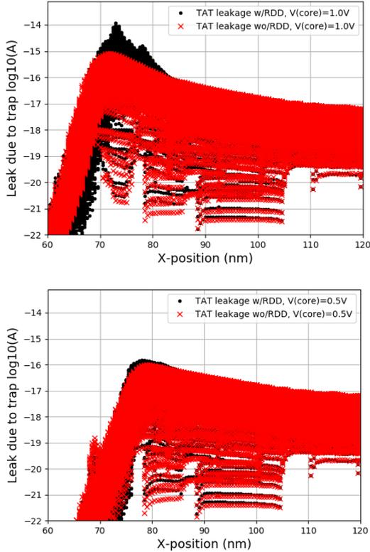
Figure 5: (top) Map of trap-related leakage against vertical position along the source/drain pillar connected to the storage capacitor, at  $V(\text{core})=1.0\text{V}$ . (bottom) The same picture, at  $V(\text{core})=0.5\text{V}$ .
