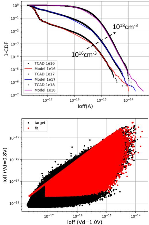
Figure 7: (top) Comparing analytically generated statistical leakage (obtained by convolution of the single trap distribution) vs TCAD-generated data for different trap densities. (bottom) The analytical generation is also able to maintain good agreement with TCAD data with respect to drain bias dependence (here shown for the case of single trap).
