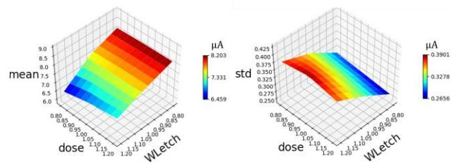
Figure 3: Mean ON-current (left) and its standard deviation (right) across the space of process variation. The plot on the right highlights the clear interplay between statistical and process variability.
