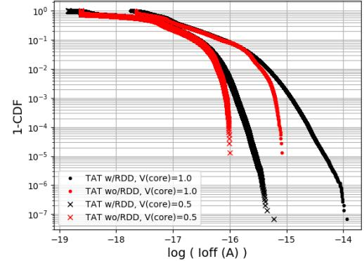
Figure 4: Complementary CDF of single trap leakage. The “w/RDD” plot represents 200 RDD configurations with ~70,000 trap evaluations per RDD configuration. The “wo/RDD” is instead obtained for a device featuring a continuous doping profile.
