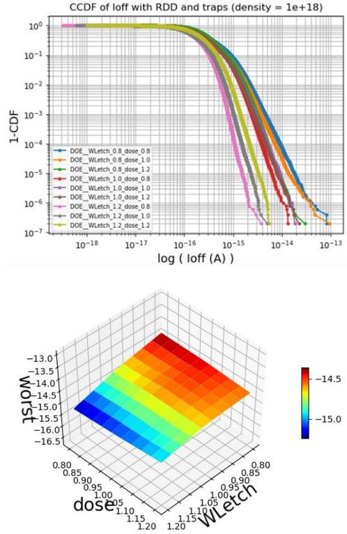
Figure 6: (top) Leakage distributions for each process condition showing  $\sim 2$  orders of magnitude difference in tail leakage for this set of experiments. (bottom) tail leakage values across different process conditions, highlighting a clear interplay between process and statistical variability also for the leakage behaviour.
