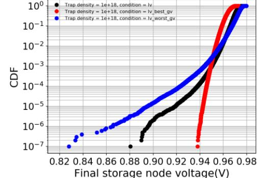
Figure 10: (top) Final storage capacitor voltage after a write and 64ms hold operation. (bottom) scatter plot of final storage node voltage after write (final\_level) vs. final storage node voltage after write and 64ms hold. The red data points represent worst tWR/best tREF process conditions, the blue represents best tWR/worst tREF conditions, and black the “typical” case.
