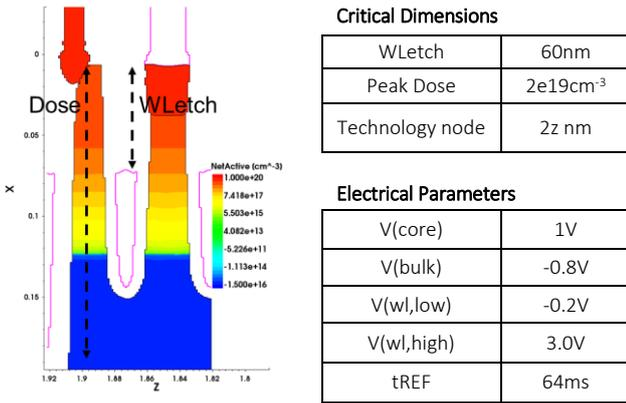
Figure 2: (left) cross-section of generated DRAM cell structure, corresponding to a 6F<sup>2</sup> technology. (right) table of critical dimensions and electrical parameters for the DRAM structure under test.
