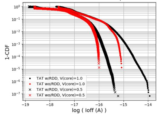
Figure 4: Complementary CDF of single trap leakage. The “w/RDD” plot represents 200 RDD configurations with ~70,000 trap evaluations per RDD configuration. The “wo/RDD” is instead obtained for a device featuring a continuous doping profile.
