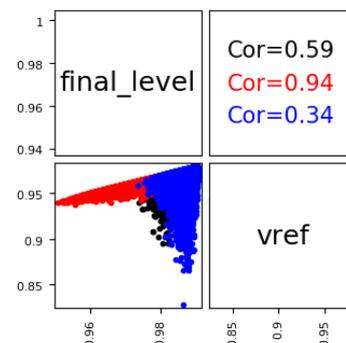
Figure 10: (top) Final storage capacitor voltage after a write and 64ms hold operation. (bottom) scatter plot of final storage node voltage after write (final level) vs. final storage node voltage after write and 64ms hold. The red data points represent worst tWR/best tREF process conditions, the blue represents best tWR/worst tREF conditions, and black the "typical" case.
