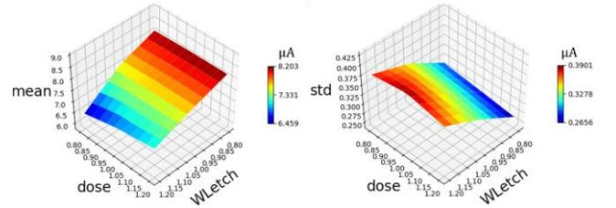
Figure 3: Mean ON-current (left) and its standard deviation (right) across the space of process variation. The plot on the right highlights the clear interplay between statistical and process variability.
