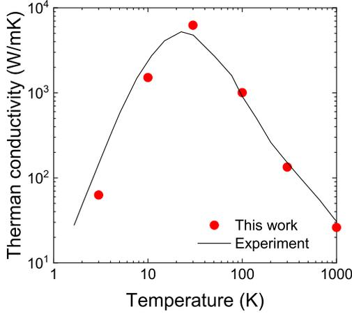
Fig. 2: Comparison of temperature-dependency of thermal conductivity of bulk Si between the simulation (dots) and experiment (line) [10].
