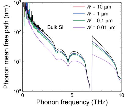
Fig. 7: Phonon mean free path for Si wire and bulk Si with respect to phonon frequency.  $\eta_{\text{side}}$  is  $1.4 \text{ nm}$ .
