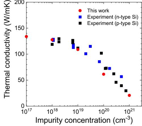
Fig. 3: Comparison of impurity concentration-dependency on thermal conductivity of bulk Si between the simulation (red) and experiment for n-type (blue) and p-type (black) [12]–[16].
