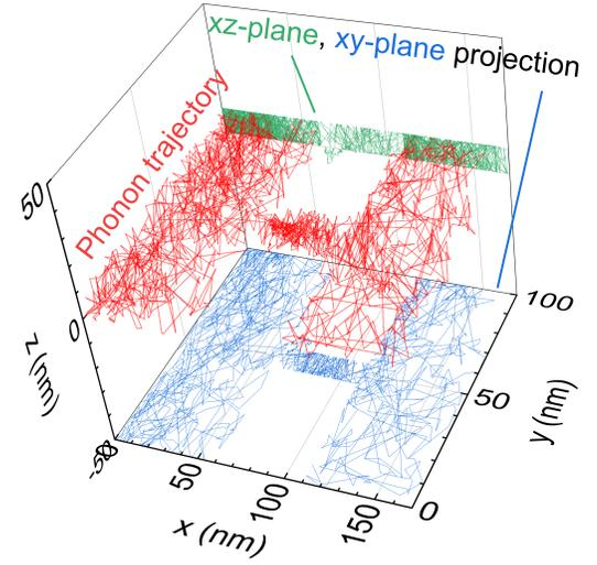
Fig. 4: Phonon trajectory in an actual Si wire structure with Si pads formed in SOI substrate.
