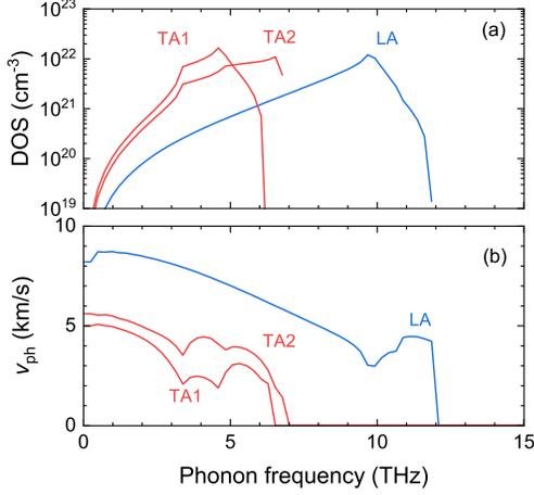
Fig. 1: Phonon frequency dependence of (a) density of states and (b) group velocity ( $v_{\text{ph}}$ ) of transverse acoustic (TA1, TA2) and longitudinal acoustic (LA) phonons calculated from the approximated dispersion curves [8].
