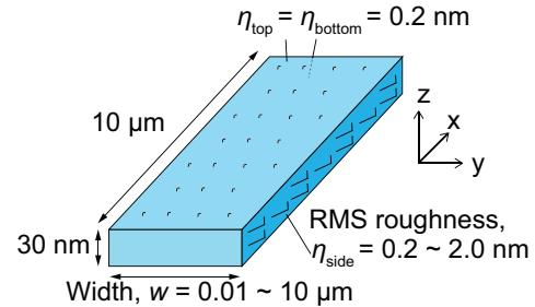
Fig. 5: Schematic of test device structure to simulate phonon mean free path.
