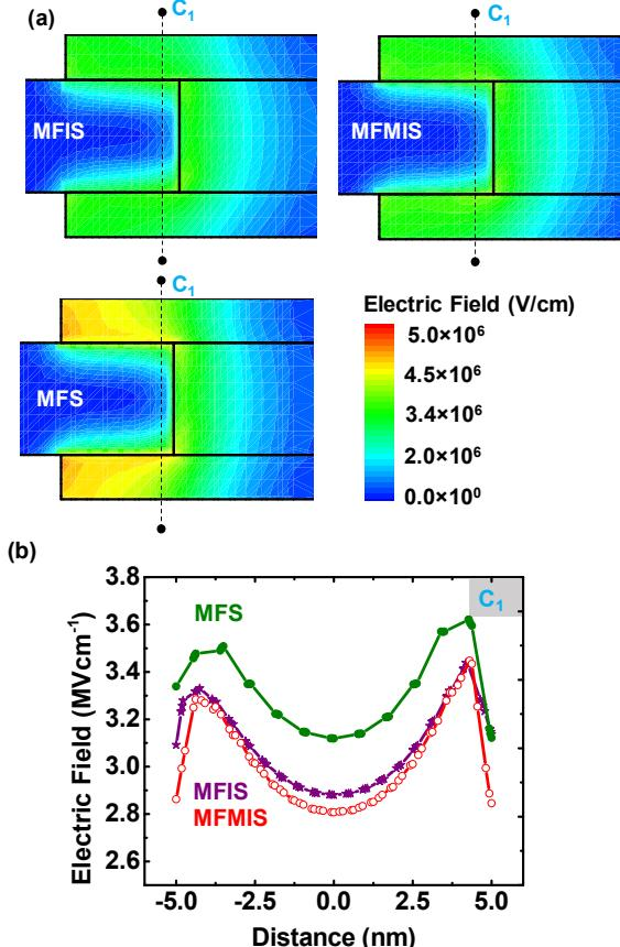
Fig. 2. (a) The electric field profile distributions and (b) its variation through n-epitaxy-source regions (along the cut-line C<sub>1</sub>) for the proposed structures of MFIS, MFMIS, and MFS based NLTFTFs.
