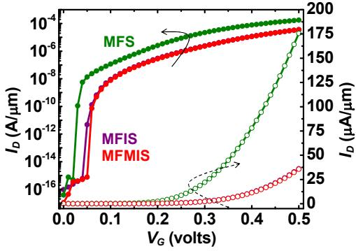
Fig. 4. The  $I_D$ - $V_G$  characteristics of MFS, MFIS and MFMIS structures at the bias level of  $V_D = V_G = 0.5 \text{ V}$  and at  $t_{FE}$  of 4 nm.
