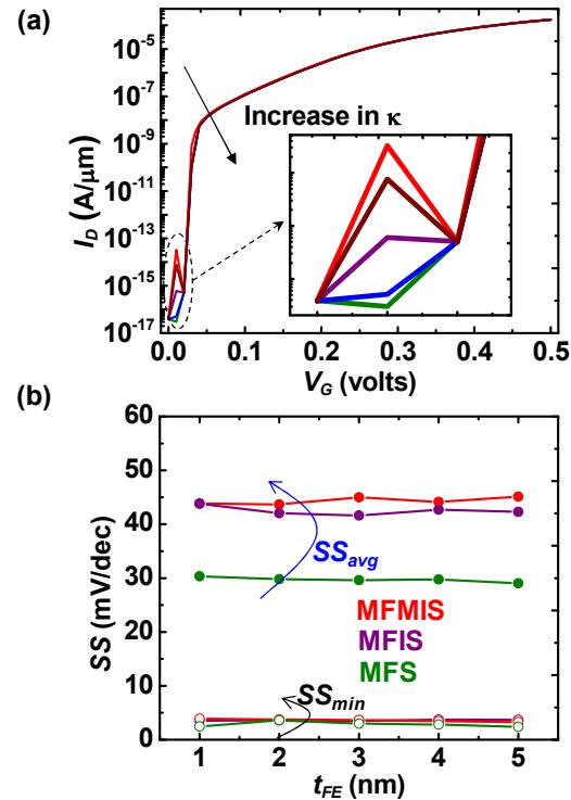
Fig. 5. (a) The extracted  $I_D$ - $V_G$  for variation in dielectric constant ( $\kappa$ ) of the  $\text{Hf}_{0.5}\text{Zr}_{0.5}\text{O}_n$  on MFS NLTFET structure. Inset shows the off-state current fluctuation for increased  $\kappa$  (red to green) at  $t_{FE}$  of 4 nm. (b) The observed  $SS_{min}$ ,  $SS_{avg}$  for the proposed structures by scaling  $t_{FE}$ .
