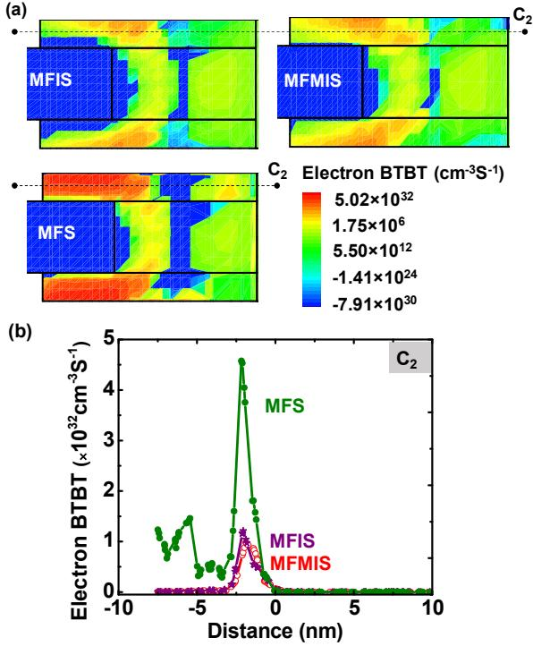
Fig. 3. (a) The distributions of electron BTBT on the proposed structures (MFIS, MFMIS, and MFS), (b) including their tunneling rate along the cut-line  $C_2$  (contributor of line tunneling).
