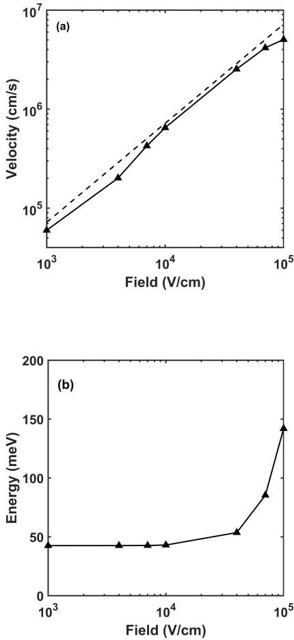
Fig. 5. (a) Velocity-field characteristics of monolayer SnSe and their corresponding (b) average energy-field plot at room temperature ( $T = 300$ K).
