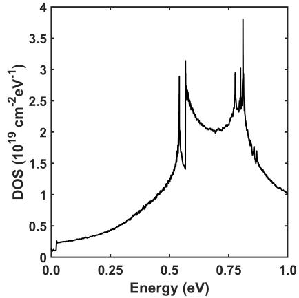
Fig. 3. Density of states plotted as a function of the electron energy with DFT calculations performed using the GGA-PBE functionals
