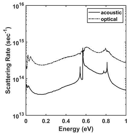
Fig. 4. The room-temperature ( $T = 300\text{K}$ ) electron scattering rates plotted as a function of the initial electron energy (average over equi-energy surfaces) with DFT calculations performed using the GGA-PBE functionals
