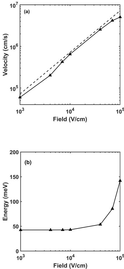
Fig. 5. (a) Velocity-field characteristics of monolayer SnSe and their corresponding (b) average energy-field plot at room temperature ( $T = 300\text{K}$ ).
