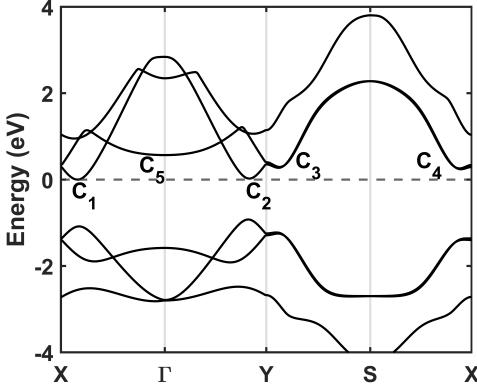
Fig. 1. Calculated band structure for monolayer SnSe along the high-symmetry directions of the first Brillouin Zone using the GGA-PBE exchange co-relational functionals
