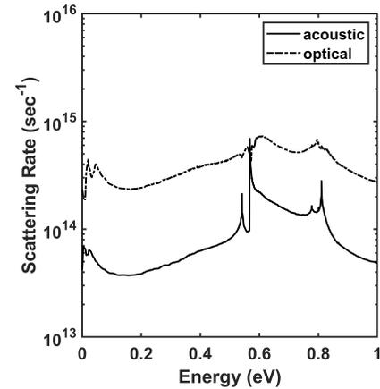
Fig. 4. The room-temperature ( $T = 300\text{K}$ ) electron scattering rates plotted as a function of the initial electron energy (average over equi-energy surfaces) with DFT calculations performed using the GGA-PBE functionals
