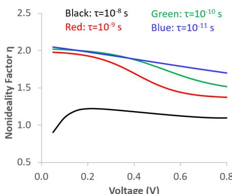
Fig. 7. NN learned non-ideality factor  $\eta(V_D)$  as a function of voltage for the pigNN results shown in Fig. 6.
