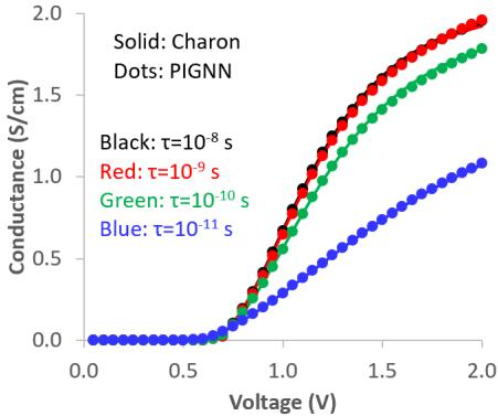
Fig. 4. Diode conductance,  $G_D(V_D)$ , vs. voltage comparison between Charon (solid) and pigNN (dots) for the same simulations as in Fig. 3.
