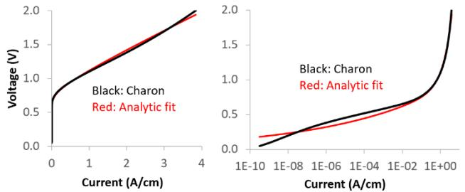
Fig. 5. Approximate voltage-current function (red line) of the Charon result for the case of  $\tau = 10^{-9}$  seconds (black line) on the linear current scale (left panel) and the log scale (right panel).
