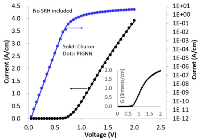
Fig. 2. Diode current-voltage comparison between Charon (solid lines) and pigNN learned results (dots) in both linear (left axis) and log (right axis) scales for the case of no SRH. Inset shows the diode conductance,  $G_D(V_D)$ , vs. voltage comparison between Charon (solid) and pigNN (dots).
