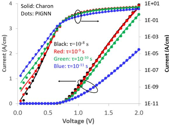
Fig. 3. Diode current-voltage comparison between Charon (solid lines) and pigNN results (dots) in both linear (left axis) and log (right axis) scales for TCAD simulations including SRH with 4 different carrier lifetimes.
