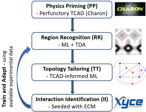
Fig. 1. Workflow of the pigNN-CMD methodology. The second and third graphs in the right column are taken from Wikipedia for illustration purpose only.
