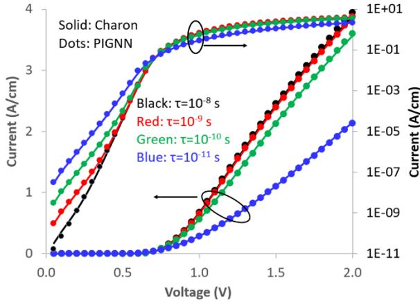
Fig. 6. Diode current-voltage comparison between Charon (solid lines) and pigNN results (dots) obtained using voltage-dependent non-ideality factors in both linear (left axis) and log (right axis) scales for TCAD simulations including SRH with four different carrier lifetimes.
