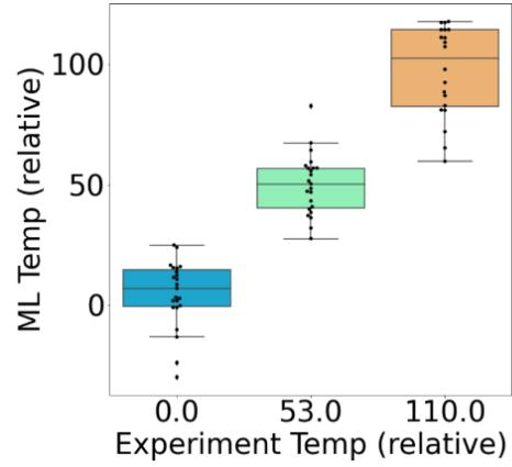
Fig. 9: Prediction of measurement ambient temperature using the machine trained with TCAD  $IV$ 's ( $\text{SNR} = 7 \text{dB}$ ).
