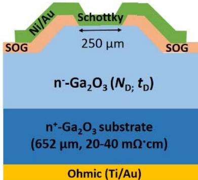
Fig. 5: Structure of the Ga<sub>2</sub>O<sub>3</sub> Schottky Diode fabricated.
