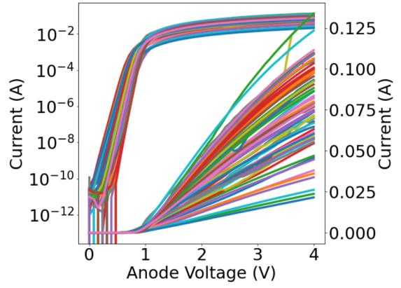
Fig. 6: 67 experimental *IV*'s of Ga<sub>2</sub>O<sub>3</sub> Schottky Diodes with variations in  $N_D$ ,  $t_D$ , and effective workfunction measured at 3 different ambient temperatures. Left: log scale. Right: linear scale
