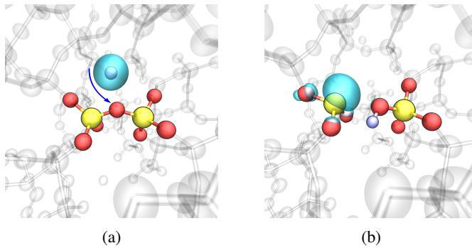
Fig. 3: Hydrogen interaction with the a-SiO<sub>2</sub> matrix (a) can lead to formation of a hydroxyl group, as well as breakage of a strained Si-O bond, resulting in a hydroxyl E' center defect (b). The blue bubbles show the spin-density associated with interstitial hydrogen and the hydroxyl E' center defect, respectively.
