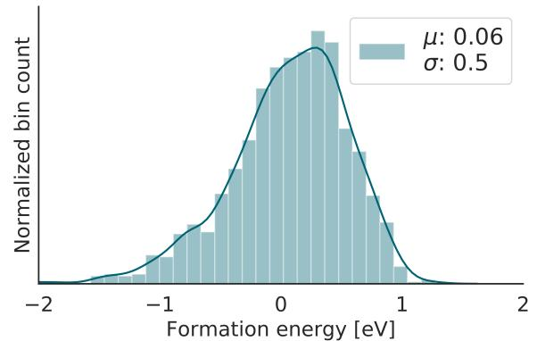
Fig. 4: Formation energies of hydroxyl E' center defects in a-SiO<sub>2</sub>, obtained with DFT calculations, together with the mean ( $\mu$ ) and standard deviation ( $\sigma$ ). The broad distribution is due to the amorphous nature of the structures.
