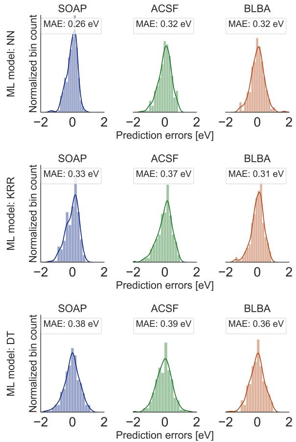
Fig. 6: Error distributions and MAE in the prediction of formation energy of hydroxyl  $E'$  center defects in a-SiO<sub>2</sub> for the different combinations of descriptors (SOAP, ACSF and BLBA) and ML models (NN, KRR and DT).
