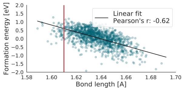
Fig. 5: Correlation between formation energies and bond-lengths. The formation energy decreases for larger bond lengths, so defects preferably form at strained Si-O bonds. The red line indicates the Si-O bond-length in alphaquartz [15].
