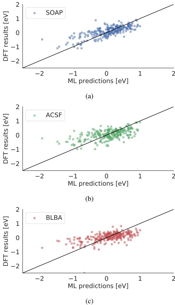
Fig. 7: Correlation between the DFT calculation results and the ML-based predictions using (a) SOAP, (b) ACSF and (c) BLBA descriptors (in all cases, combined with a neural network). All descriptors perform similarly. However, SOAP shows a slightly better correlation in general, particularly for negative values.
