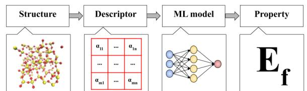
Fig. 1: Workflow to predict a property from an atomistic structure. The structure must be represented by a descriptor. Then, a ML model can be trained and subsequently be used to predict the desired property in new atomistic structures.
