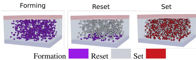
Fig. 4: Ion vacancy distributions for TiN/SiO<sub>x</sub>/TiN structure, during the forming, reset (overlapping of forming and reset ion vacancies) and set (overlapping of reset and set ion vacancies) processes.
