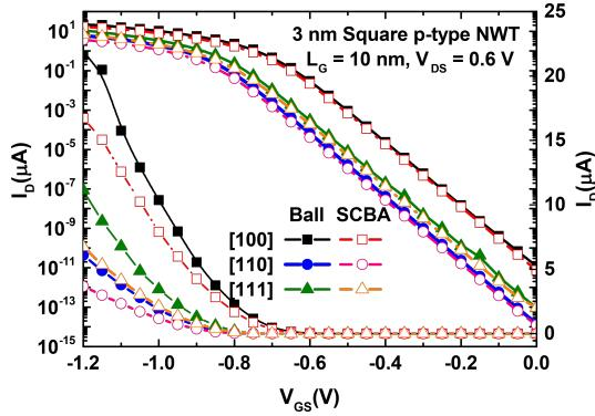
Fig. 7:  $I_D$  vs.  $V_{GS}$  characteristics for p-type square 3 nm Si NWTs considering the most common crystallographic orientations ([100, 110, 111]) with coherent and dissipative transport. The results have been simulated making use of the mode-space full-band quantum transport solver included in NESS by combining a six-band  $k \cdot p$  Hamiltonian and the existing NEGF module.
