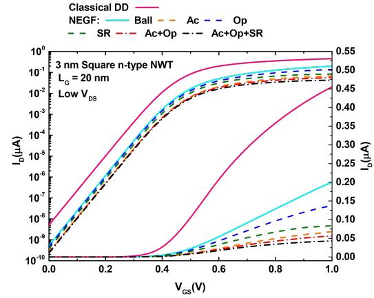
Fig. 2:  $I_D$  vs.  $V_{GS}$  characteristics for n-type square 3nm Si NWTs with  $L_G=20\text{nm}$  using the classical DD and the NEGF modules, assuming ballistic and dissipative transport with acoustic (Ac), g-type optical (Op) phonon and surface roughness (SR) scattering mechanisms
