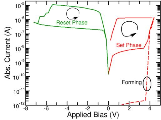
Fig. 5: Simulation characteristic of a bipolar SiO<sub>x</sub> based RRAM device. The compliance current of 1μA was enforced in the simulation.
