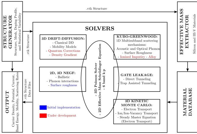
Fig. 1: Flowchart of NESS detailing its modular structure.
