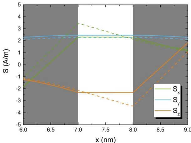
Figure 3. Spin accumulation across the middle layer, with magnetization along  $z$  in the FL and along  $x$  in the RL. The dashed lines use the same value for  $D_S$  in TB and  $D_e$  in the FL/RL, while solid lines use a very high value of  $D_S$ .
