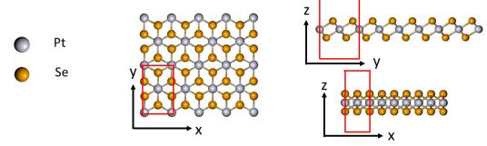
Fig. 2. Orthorombic unit cell of the 1T phase monolayer PtSe<sub>2</sub>.
