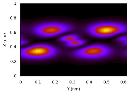
Fig. 4. Contourplot of the cross section of the electron density at an abscissa  $x$  corresponding to the center of the orthorombic unit cell. Colors are in arbitrary units.
