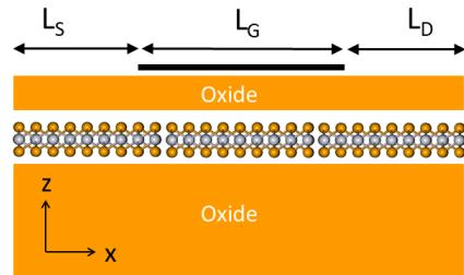
Fig. 6. Sketch of the single-gate monolayer  $\text{PtSe}_2$  FET.
