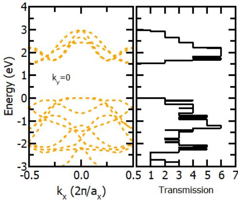
Fig. 5. Bandstructure of an infinitely-long monolayer  $\text{PtSe}_2$  and the corresponding transmission probability obtained with the Hamiltonian in the reduced basis consisting of unit-cell-restricted Bloch states.  $k_y = 0$ .
