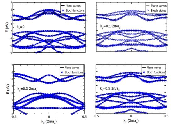
Fig. 3. Bandstructure of the monolayer PtSe<sub>2</sub> for various  $k_y$  values computed with (circles) the Bloch function basis and (lines) the PW basis.
