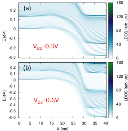
Fig. 8. LDOS computed for (a)  $V_{DS}=0.3$  V and (b)  $V_{DS}=0.6$  V and for  $V_{TG} = 0.8$  V. The transverse wave-vector is  $k_y = 0.1 \times 2\pi/a_y$ .
