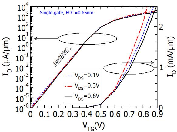
Fig. 7. Transfer characteristics of the monolayer PtSe<sub>2</sub> FET for  $V_{DS}=0.1$ , 0.3 and 0.6 V.
