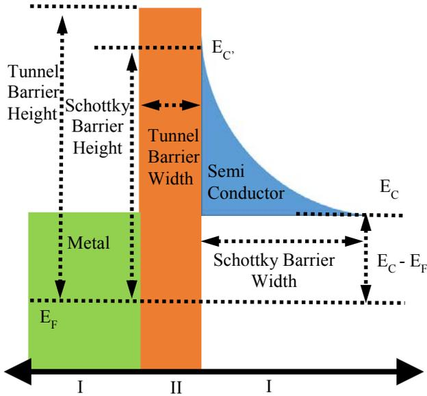
Figure 1: Schematic of different types of barriers in the carrier transport at the metal-2D materials interface.
