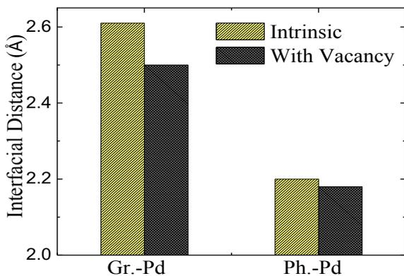
Figure 2: Defect Engineering (Creating Vacancy) reduces interfacial distance significantly (2.61 Å to 2.50 Å) for Graphene-Pd interface but it doesn't have significant impact on the interfacial distance (2.20 Å to 2.18 Å) of the Phosphorene-Pd interface.
