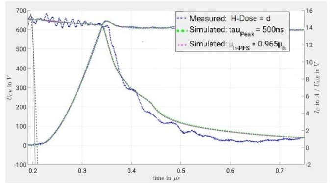
Fig. 12: Comparison of the two simulated turn-off transients based on adjusted empirical models and the measured turn-off transients of the FS devices at room temperature.
