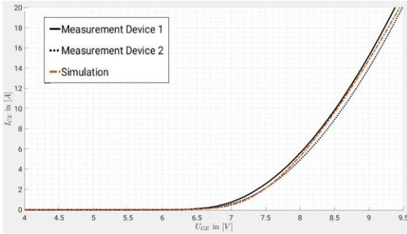
Fig. 5: Measured and calibrated simulated transfer characteristic as obtained after adjusting the density of oxide charges and the contact resistance.
