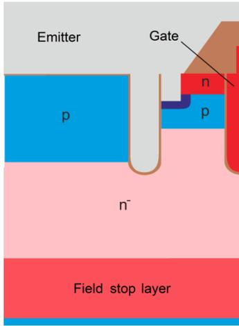
Fig. 2: Two-dimensional TCAD model of the IGBT trench cell under test.
