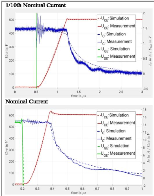
Fig. 6: Comparison of simulated and measured turn-off transients of the reference DUT at room temperature.
