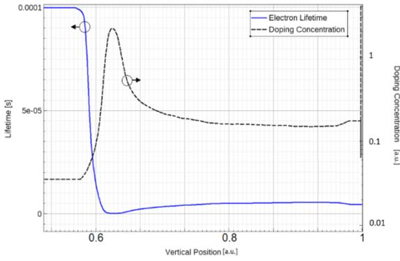
Fig. 9: Carrier lifetime profile (blue) as used for simulation. It has been generated on the basis of spreading resistance measurements of the doping concentration and the relation  $\tau = 1/(C_{\text{fact}} \cdot N_{D,\text{SRP}})$ .
