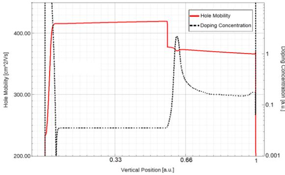
Fig. 10: Hole mobility profile (red) as used for simulation. The mobility along the implantation path is reduced by 5%.
