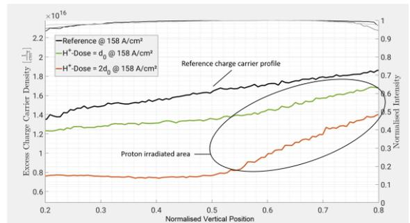
Fig. 8: FCA measurements at room temperature on the FS DUTs reveal that the charge carrier gradient along the implantation path becomes steeper with increasing hydrogen implantation dose.
