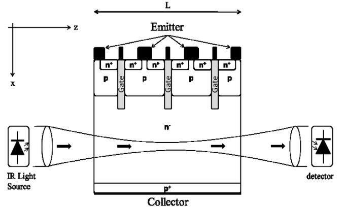
Fig. 3: Schematic drawing of the optical beam path in free-carrier absorption experiments.
