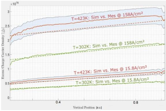
Fig. 4: Measured (solid) and simulated (dashed) excess charge carrier profiles in the reference DUT at room temperature (green) and 150°C (red).
