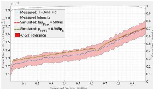
Fig. 11: Measured excess charge carrier density compared to simulations with adjusted model parameter for room temperature.
