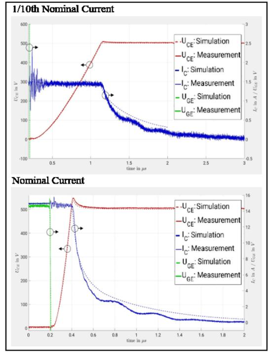
Fig. 7: Comparison of simulated and measured turn-off transients of the reference DUT at T=150°C.
