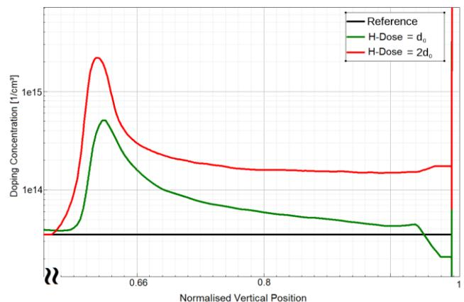
Fig. 1: Implanted hydrogen donor profiles and background doping of the reference device obtained from spreading resistance measurements.
