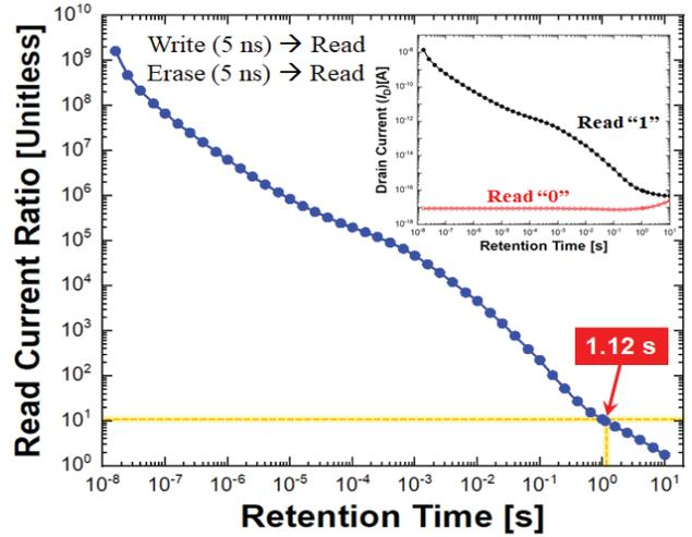
Fig. 5. Read-1/read-0 current ratio as a function of time. Retention time as long as 1.12 s is obtained by a presumable reference current ratio of  $10^1$ . The inset shows the raw read currents.
