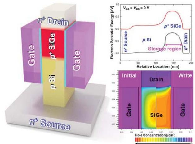
Fig. 1. Schematic of the SiGe QW 1T DRAM cell. Insets for off-state energy-band diagram (upper) and hole distributions at off-state (lower left segment) and right after a write operation is completed (lower right).
