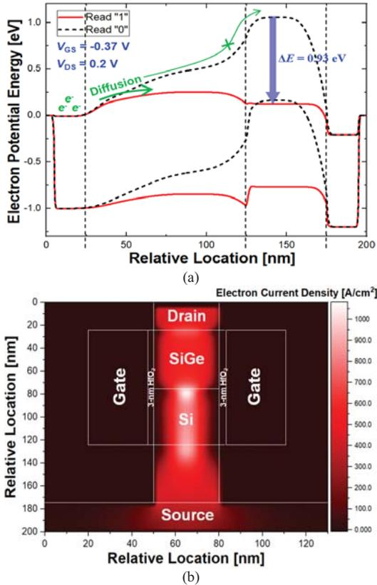
Fig. 3. Read operation characteristics. (a) Energy-band diagrams at read operations for state 0 (upper) and 1 (lower). (b) Electron current density contour under the read-1 operation condition.
