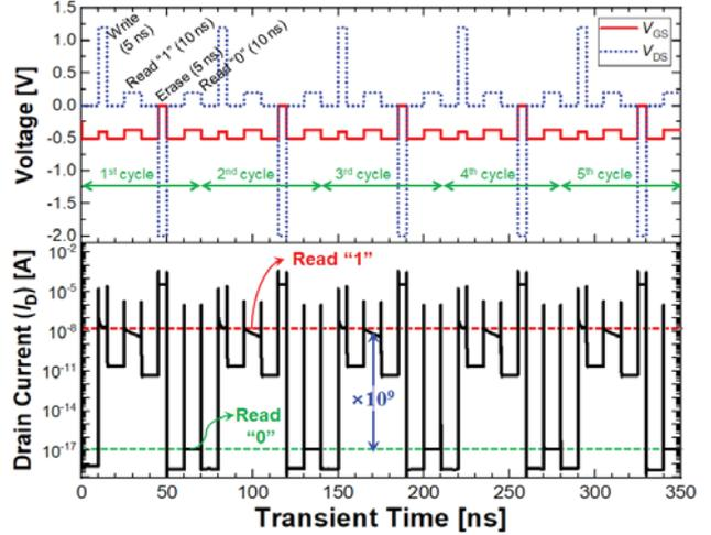
Fig. 4. Transient operation characteristics of the Si<sub>0.7</sub>Ge<sub>0.3</sub> QW 1T DRAM over 5 cycles where a single cycle consists of 8 operations (write 1/hold/read 1/hold/write 0/hold/read 0/hold).
