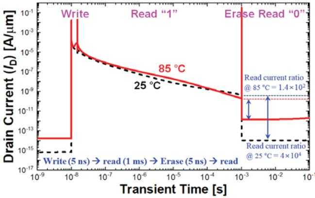
Fig. 6. Temperature dependence of drain currents in the respective operation regions at 25 °C and 85 °C. Even under the harsher temperature condition, current ratio is maintained to be  $> 10^2$ .
