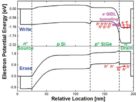
Fig. 2. Energy-band diagrams. Program (upper) and erase (lower) operations.
