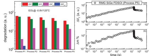
Fig.12. EOL  $\Delta V_T$  at operating conditions and underlying subcomponents for Ge% and N% at changes in FDSOI devices.
