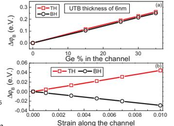
Fig.23. (a) Channel Ge% impact on TH and BH bands. (b) Uniaxial compressive strain impact on TH and BH bands.
