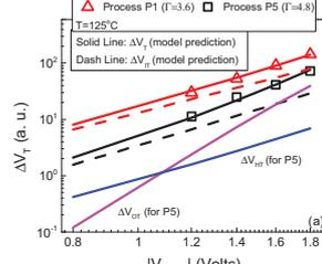
Fig.11.  $V_{GSTR}$  dependence of fixed time degradation for Si and SiGe devices. The  $\Delta V_{IT}$  (dash line) at operating voltage is close to  $\Delta V_T$ .
