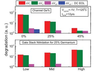
Fig.19. EOL  $\Delta V_T$  under operating conditions and underlying subcomponents for different Ge% (top) and different  $N\%$ .
