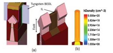
Fig.27. (a) TCAD [13] structure used for Si and SiGe FinFET simulation. (b) Hole density profile in channel Fin. Proper mechanism for Si-H bond dissociation (Fig.2) is used.
