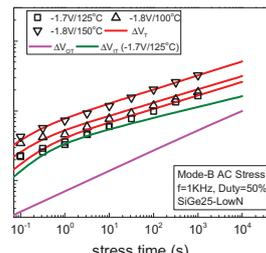
Fig.16. Prediction of stress kinetics in RMG SiGe p-FinFET during AC stress for different  $V_{GSTR}$  and  $T$ . Subcomponents for the lowest dataset are shown.
