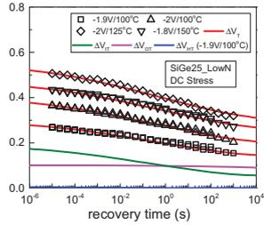
Fig.15. Prediction of recovery kinetics in RMG SiGe p-FinFET after DC stress for different  $V_{GSTR}$  and  $T$ . Subcomponents for the lowest dataset are shown.
