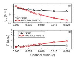
Fig.26. Mechanical strain dependence of (a)  $\Delta V_T$  pre-factor  $k_{FIT}$  and (b) tunneling parameter ( $\Gamma_0$ ). FinFETs shows steeper strain dependence due to (110) sidewall.
