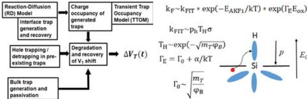
Fig.1. Schematic of a comprehensive NBTI modeling framework consisting of uncorrelated  $\Delta V_{IT}$ ,  $\Delta V_{HT}$  and  $\Delta V_{OT}$  components.
