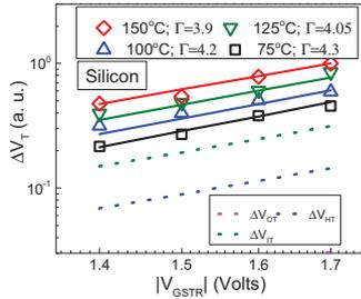
Fig.18. Model prediction of measured fixed time  $\Delta V_T$  versus  $V_{GSTR}$  at different  $T$  for Si and SiGe RMG p-FinFETs with different  $N\%$ . VAF decreases with  $T$ . VAF (iso- $T$ ) increases with increase in Ge% and reduces with increase in  $N\%$ .
