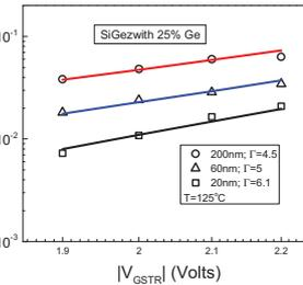
Fig.21. Prediction of  $\Delta V_T$  as a function of  $V_{GSTR}$  for different channel length.
