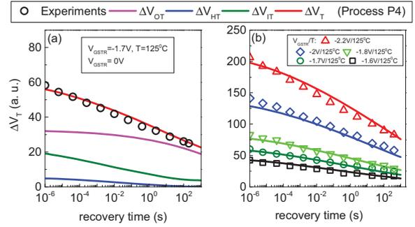
Fig.5 (a) Time evolution of UF measured  $\Delta V_T$  for recovery after DC stress, with model prediction and different subcomponents at fixed  $V_{GSTR}$  and T. (b) Model prediction of UF measured  $\Delta V_T$  for recovery after DC stress for multiple  $V_{GSTR}$ .
