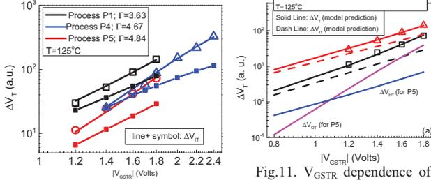
Fig.10. Model prediction of fixed time  $\Delta V_T$  for different processes.  $\Delta V_{IT}$  shown by line + symbols.
