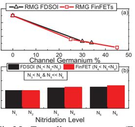
Fig.25. Tunneling parameter ( $\Gamma_0$ ) as a function of (a) channel Ge% and (b)  $N\%$  in IL.  $\Gamma_0$  reduces with Ge% due to change in  $\phi_B$ , but weakly depend on gate stack  $N\%$ .
