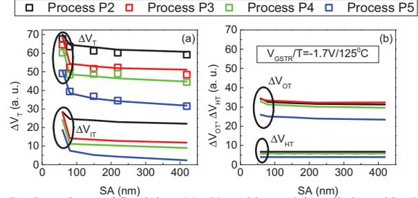
Fig.9. SA dependence of fixed time (a)  $\Delta V_T$  and its model prediction with  $\Delta V_{IT}$  subcomponent and (b)  $\Delta V_{HT}$  and  $\Delta V_{OT}$  subcomponents, for DC stress in FDSOI having different processes. SA induced variation is due to changes in  $\Delta V_{IT}$ .
