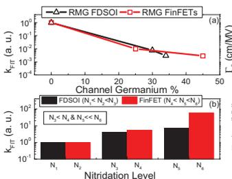
Fig.24.  $\Delta V_T$  pre-factor as a function of (a) channel Ge% and (b)  $N\%$  in IL. It reduces with higher Ge% but increases with higher  $N\%$ .
