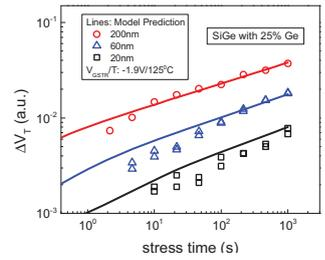
Fig.20. Prediction of  $\Delta V_T$  time kinetics for different channel length at fixed  $V_{GSTR}/T$ .  $\Delta V_T$  reduces with reduction in  $L$ .
