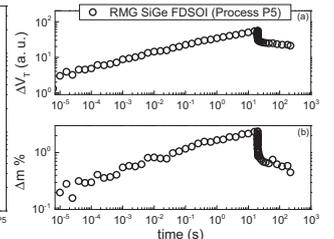
Fig.13. Measured stress-recovery time kinetics for (a)  $\Delta V_T$ , and (b) body coefficient (m).
