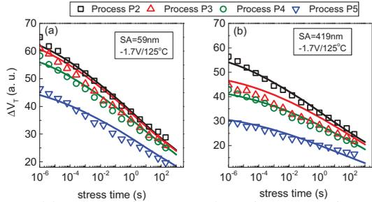
Fig.8. Model prediction of UF measured  $\Delta V_T$  for recovery after DC stress for different Ge% in the channel and N% in the gate stack for (a) SA=59 and (b) SA=419.
