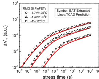
Fig.28. TCAD prediction of  $\Delta V_T$  stress time kinetics (extracted from analysis of p-FinFETs) at different  $V_{GSTR}$  and  $T$  for Si (left) and SiGe (right) p-FinFETs.
