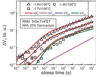
Fig.14. Prediction of stress kinetics in RMG SiGe p-FinFET during DC stress for different  $V_{GSTR}$  and  $T$ . Subcomponents for the lowest dataset are shown.
