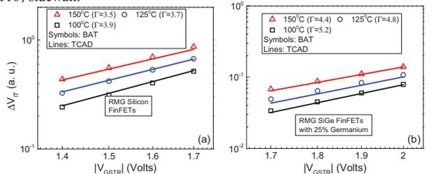
Fig.29. TCAD prediction of fixed time  $\Delta V_T$  (extracted from measured  $\Delta V_T$ ) as a function of  $V_{GSTR}$  at different  $T$ , for (a) Si channel and (b) SiGe channel with 25% Germanium RMG FinFETs. SiGe devices show higher VAF and larger  $T$  impact of VAF due to polarization (see Fig.2).
