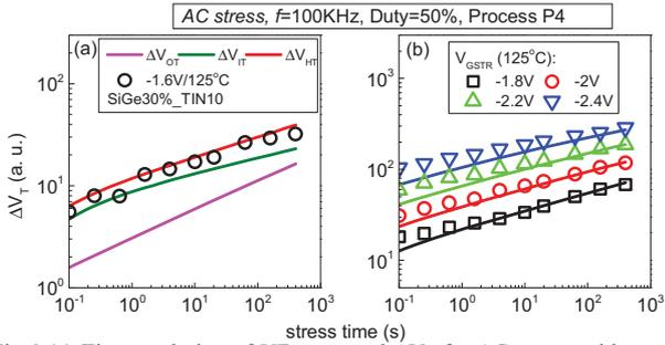
Fig.6 (a) Time evolution of UF measured  $\Delta V_T$  for AC stress, with model prediction and different subcomponents at fixed  $V_{GSTR}$  and T. (b) Model prediction of UF measured  $\Delta V_T$  for AC stress for multiple  $V_{GSTR}$ .
