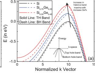
Fig.22. Simulated top and bottom hole (TH and BH) bands for Si and SiGe showing strong Ge% impact on the barrier  $\phi_B$ .
