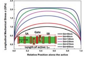
Fig.3. Stress profiles along the active for various STI to Gate length (SA).
