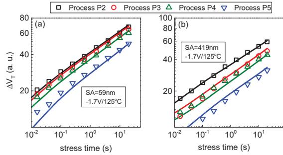
Fig.7. Model prediction of UF measured  $\Delta V_T$  for DC stress for different Ge% in the channel and N% in the gate stack for (a) SA=59 and (b) SA=419.  $\Delta V_T$  reduces with increases in SA.
