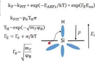
Fig.2. Schematic of Si-H bond dissociation at the channel/IL interface. Inversion layer holes tunnel into interfacial Si-H bonds aided by the oxide electric field ( $E_{OX}$ ).
