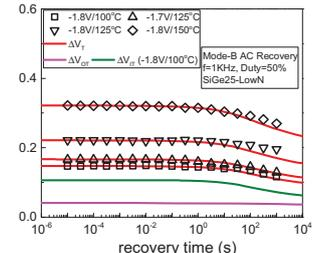
Fig.17. Prediction of recovery kinetics in RMG SiGe p-FinFET after AC stress for different  $V_{GSTR}$  and  $T$ . Subcomponents for the lowest dataset are shown.
