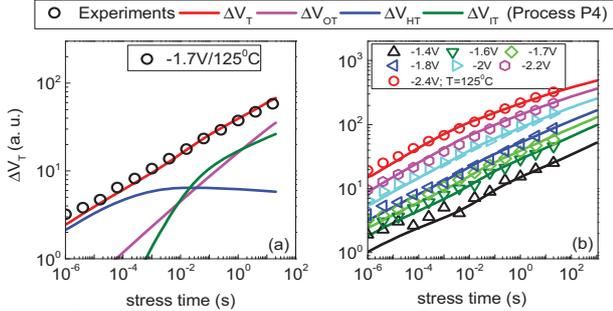
Fig.4 (a) Time evolution of UF measured  $\Delta V_T$  for DC stress, with model prediction and different subcomponents at fixed  $V_{GSTR}$  and T. (b) Model prediction of UF measured  $\Delta V_T$  for DC stress for multiple  $V_{GSTR}$ .
