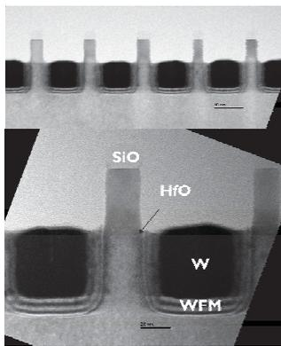
Fig. 6. Gate W / W filled metal Etch Back
