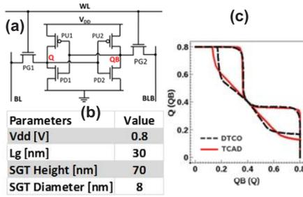
Fig. 2. (a) bit cell schematics; (b) Design Guide; (c) butterfly curve and SNN
