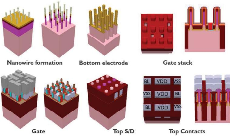
Fig.9. Sentaurus Process Explorer flow following closely the actual flow detailed in Fig.3.
