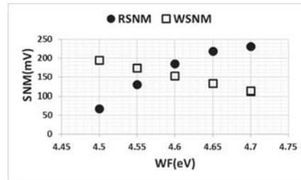
Fig. 5. RSNM & WSNM vs WF variations
