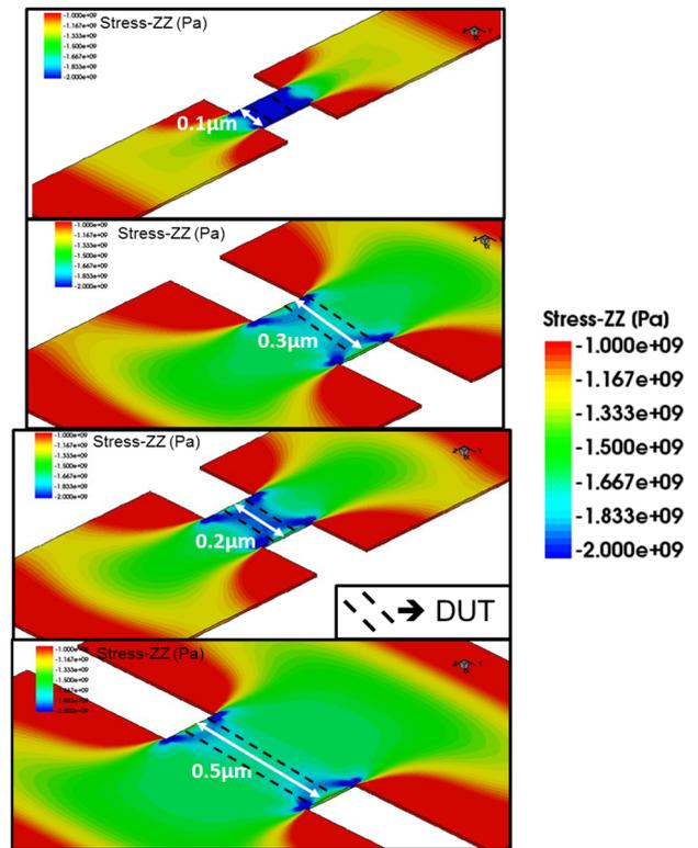
Figure 10: longitudinal stress profile obtained by 3D TCAD on Continuous-RX structure with Wfactor =2
