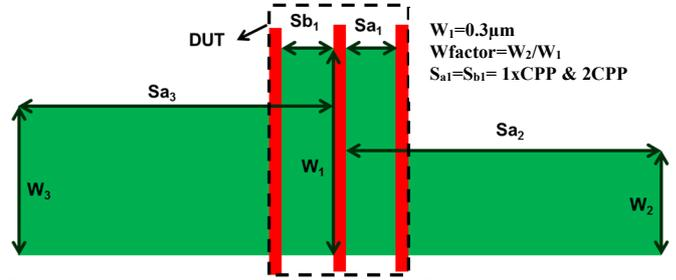
Figure 7: test structure to monitor ContinuousRX structure performance with the definition of variable parameter.
