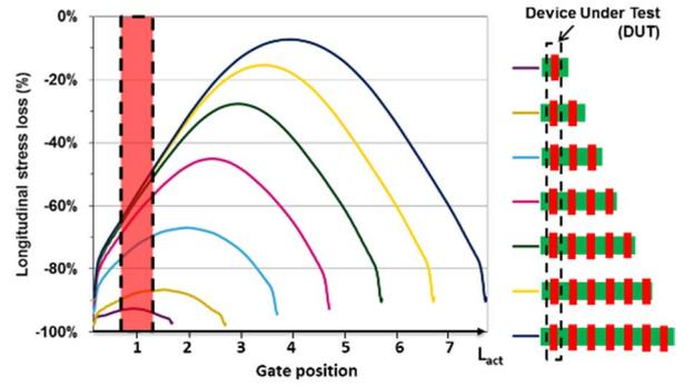
Figure 6: Longitudinal stress loss variation as a function of active length evidencing that, in dissymmetric case, the shorter side of active region is driving the performance (TCAD until full STI process).
