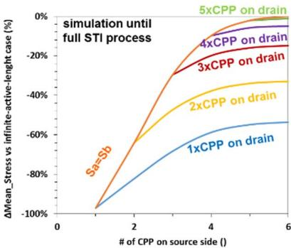
Figure 5: TCAD variation of mean longitudinal stress under the gate normalized by infinite active length case as a function of source length in symmetric & dissymmetric cases.
