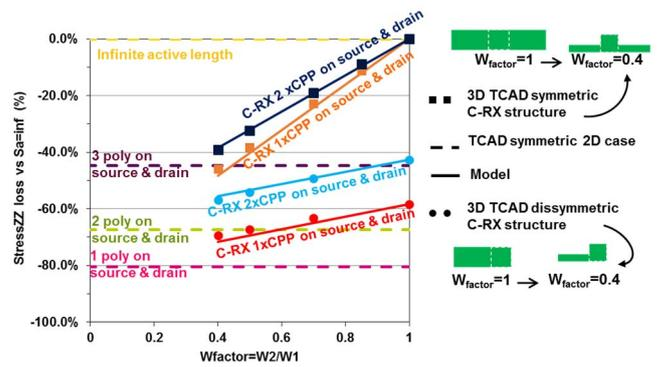
Figure 9: longitudinal stress variation vs infinite active length case (Sainf) for variation of Wfactor= $W_2/W_1$  obtained by TCAD & analytical model.
