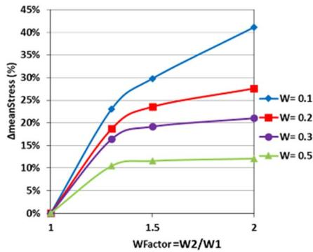
Figure 11: Longitudinal stress improvement compare to infinite active length case brought by Continuous-RX structure with Wfactor>1
