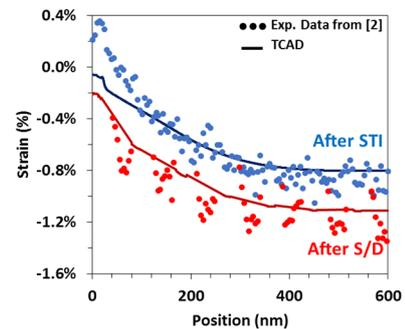
Figure 1: Strain in active region as a function of the distance with STI edge obtained by NBD measurement from [2] and simulation; blue: after STI patterning & red: after raised S/D
