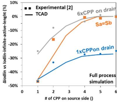
Figure 4: Variation of Iodlin ( $I_d$  at  $V_d=50mV$  &  $V_g-V_t=500mV$ ) normalized by infinite active length case as a function of source length in symmetric & dissymmetric cases.
