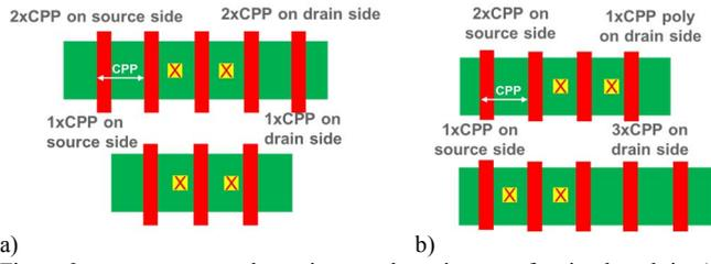
Figure 3: test structures schematic to evaluate impact of active length in a) Symmetric case b) dissymmetric case.
