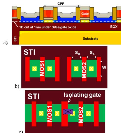
Figure 2: a) Half TCAD structure used to evaluate active length impact on performance b) classical active region c) ContinuousRX
