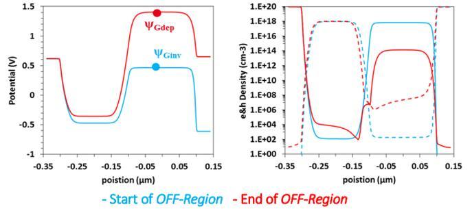
Figure 6: Potential and carrier densities from cathode to anode during *OFF-Region*
