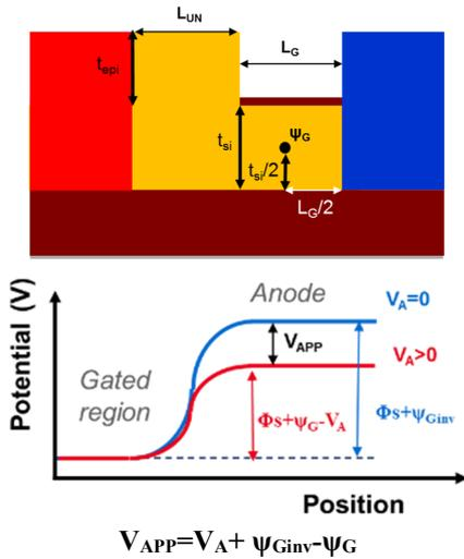
Figure 11: Z<sup>2</sup>-FET modeling parameters and applied voltage  $V_{APP}$  evaluation.
