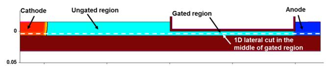
Figure 1: *Z<sup>2</sup>-FET* structure simulated with device TCAD including a representation of the 1D cut from cathode to anode used to analyse DC behavior.
