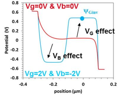
Figure 5: Potential from cathode to anode during *initialization*
