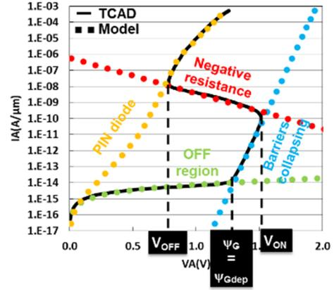
Figure 13: Z<sup>2</sup>-FET analytical models validation by DC TCAD.
