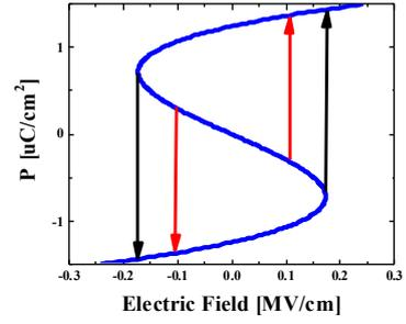
Fig. 2  $P$ - $E$  relationship of FE material based on Landau theory. The negative  $dP/dE$  part is unstable in a single FE capacitor. With parallel connection with semiconductor, the negative region will become stable and be used to achieve negative capacitance effect.
