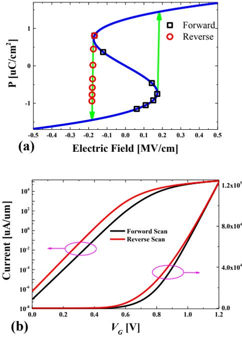
Fig. 5. (a) Operation path for Si nMOSFETs with gate length of 14 nm. (b)  $I_D$ - $V_G$  characteristics for Si nMOSFETs with gate length of 14 nm. The gate voltage range is 0.0 V to 1.2 V.
