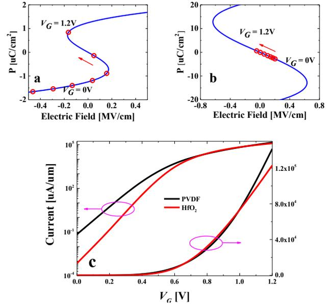
Fig. 6. (a) Operation path for Si nMOSFETs with FE material PVDF. (b) Operation path for Si nMOSFETs with FE material Si doped HfO<sub>2</sub>. (c)  $I_D$ - $V_G$  characteristics for Si nMOSFETs with PVDF and HfO<sub>2</sub>. Gate length = 6nm. Gate bias is applied from 0.0 V to 1.2 V.
