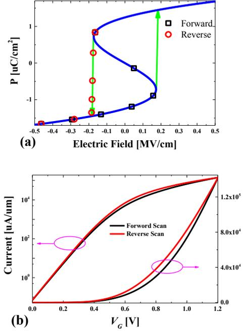
Fig. 4. (a) Operation path for Si nMOSFETs with gate length of 6 nm. (b)  $I_D$ - $V_G$  characteristics for Si nMOSFETs with gate length of 6 nm. The gate voltage range is 0.0 to 1.2 V.
