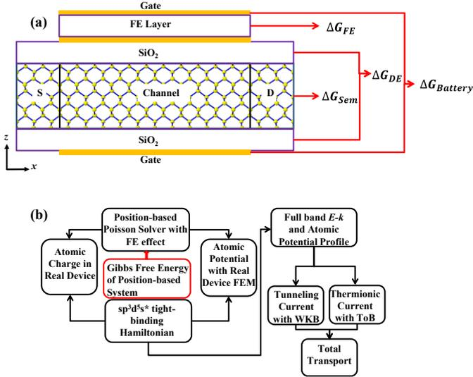
Fig. 1. (a) Cross-sectional view of device structure investigated in this work with atomic channel structure. The components of total Gibbs free energy are also indicated. (b) Procedures of the self-consistently solved atomic device performance simulation. Gibbs free energy calculation is involved in the Poisson Solver.
