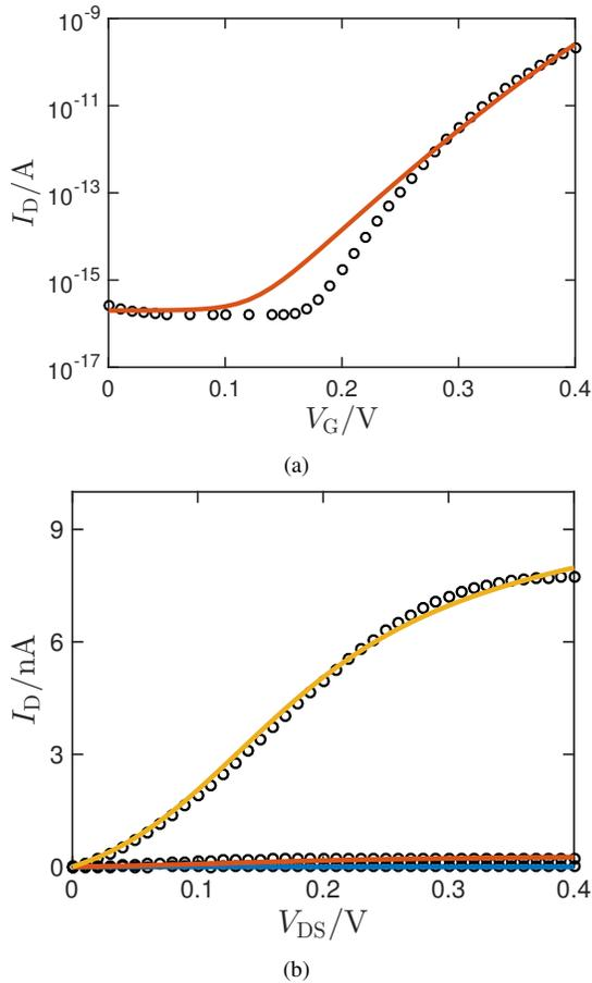
Figure 6. Comparison between the numerical device simulation results (symbols) and the compact model (solid line) for a single tube RT-FET in *nLP-mode*: (a) transfer characteristic for  $V_{DS} = 0.4$  V; (b) output characteristic for  $V_{GS} = 0.2$  V, 0.4 V and 0.6 V.
