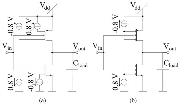
Figure 7. Schematic of the inverter in (a) LP-mode and (b) HP-mode configuration.
