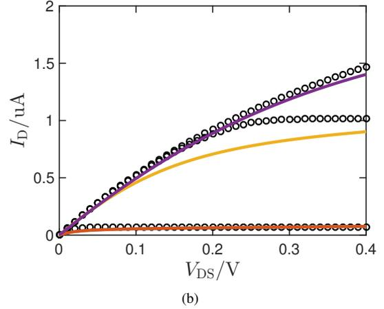
Figure 5. Comparison between the numerical device simulation results (symbols) and the compact model (solid line) for a single tube RT-FET in nHP-mode: (a) transfer characteristic for  $V_{DS} = 0.4 \text{ V}$  and  $0.8 \text{ V}$ ; (b) output characteristic for  $V_{GS} = 0.2 \text{ V}$ ,  $0.4 \text{ V}$  and  $0.6 \text{ V}$ .
