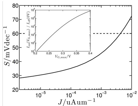
Figure 2. Sub-threshold slope  $S$  as function of the current per gate width for a tube density of  $60 \mu\text{m}^{-1}$ . The inset shows the ratio between the on and off current of the RT-nanoFET in nLP mode. The onset of leakage limits a useful control-gate supply to  $V_{G,\text{max}} > 0.2$  V at  $V_{DS} = 0.4$  V.
