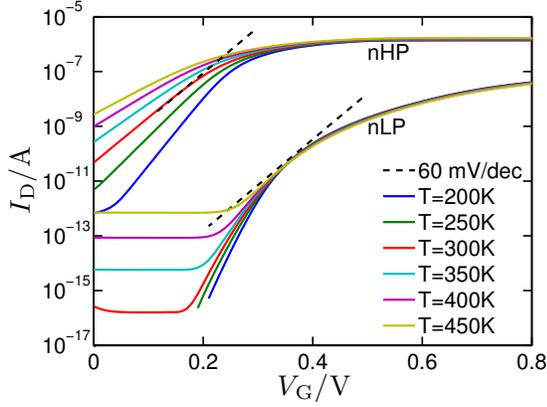
Figure 4. Temperature dependence of the transfer characteristics in LP and HP mode.
