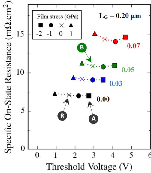
Fig. 9. Comparison of the trade-off between  $V_{\text{TH}}$  and  $R_{\text{ON}}$  for  $\sigma_{\text{SiN}}$  ranging from  $-2$  GPa to  $1$  GPa and  $x_{\text{buffer}}$  ranging from  $0.00$  to  $0.07$ .
