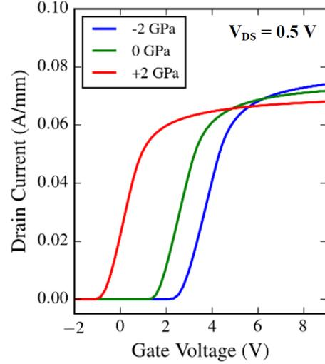
Fig. 7. Transfer characteristics  $I_{DS}(V_{GS})$  of the simulated pGaIn gate HEMTs showing the impact of  $\sigma_{SiN}$ . The device embedding highly tensile SiN film is no longer normally-OFF due to the large negative  $V_{TH}$  shift.
