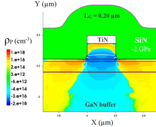
Fig. 4. Two-dimensional distribution of the polarization-induced charge density ( $\rho_P$ ) generated in the III-N heterostructure consequently of stressed nitride layer deposition.  $\sigma_{\text{SiN}} = -2$  GPa,  $L_G = 0.2 \mu\text{m}$ .
