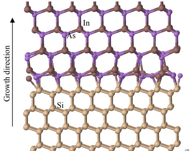
**Fig. 2: Unit cell of the InAs/Si interface obtained by geometrical optimization of the first two layers of InAs.**
