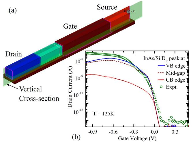
**Figure 1: (a) Device structure of a lateral nanowire TFET (b)  $I_D$ - $V_{GS}$  curves simulated with three different energetic positions of the  $D_{it}$  peak in the InAs gap. Figures taken from [2].**
