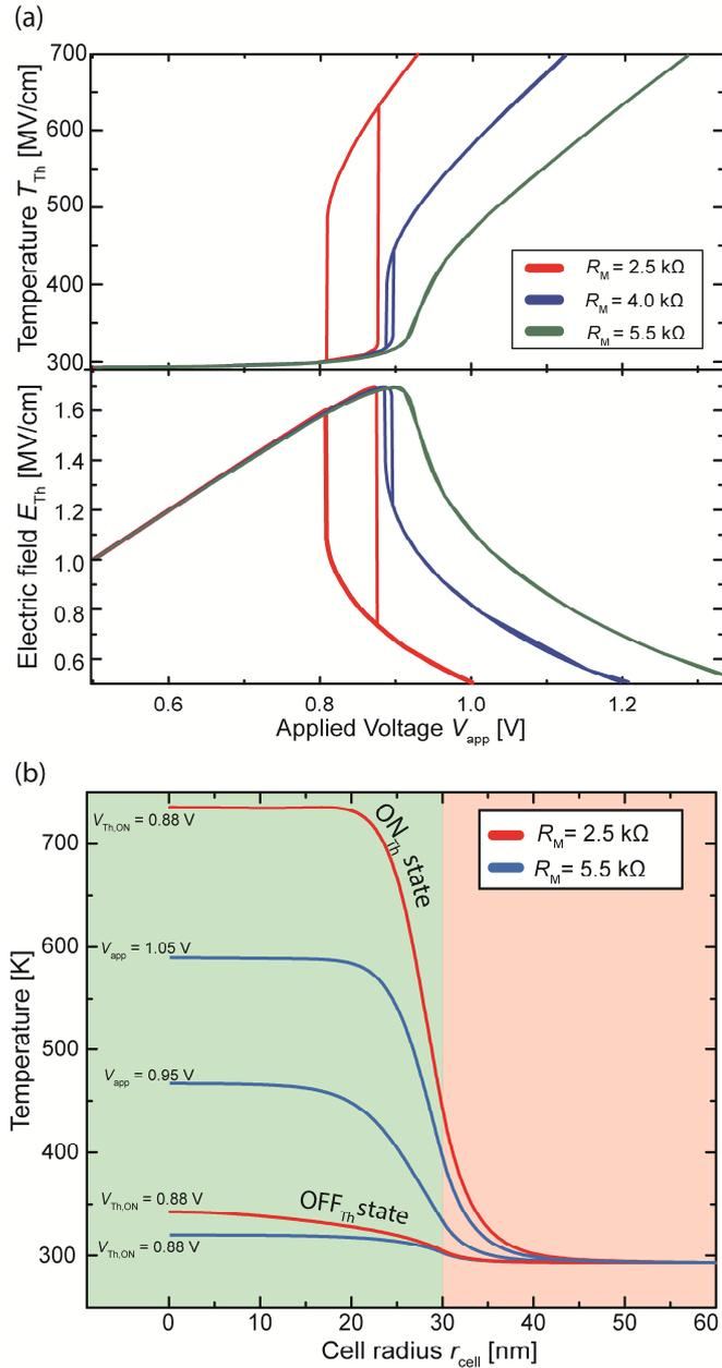
Fig. 3. (a) Average temperature and electric field in the threshold switching region for three different memristive resistances. (b) Radial temperature calculations in the axial center of the threshold region for the case of an abrupt FTTR-type threshold switching (red) at the onset voltage  $V_{Th,ON}$  for the OFF<sub>Th</sub> and ON<sub>Th</sub> state. For the resistance of 5.5 k $\Omega$  (blue) with a continuous  $I-V$  curve several radial temperature distributions are shown.
