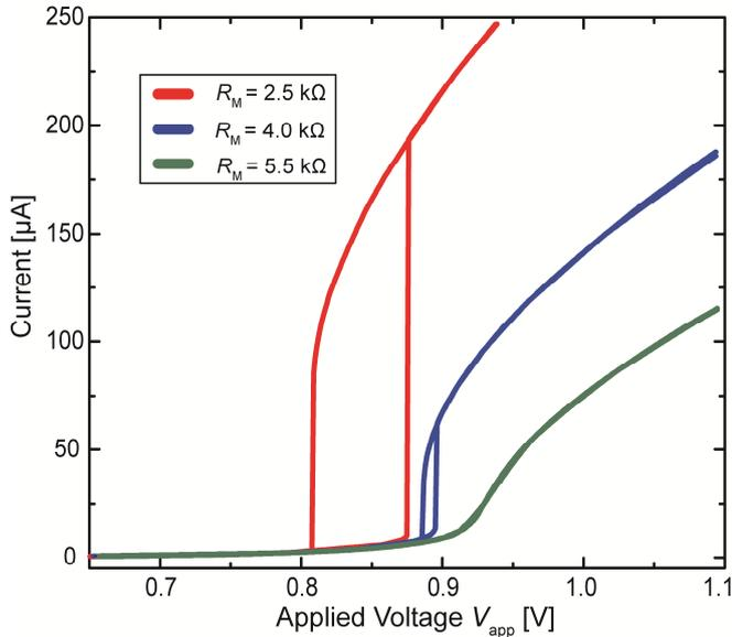
Fig. 2.  $I$ - $V$  characteristics of the simulated FTTR type threshold switching using different memristive resistances. The red  $I$ - $V$  curve with the lowest memory resistance shows a significant higher resistance jump and a greater hysteresis. With increasing resistance of the memristive part the resistance jump and the hysteresis decreases until the abrupt threshold switching vanishes (green curve).
