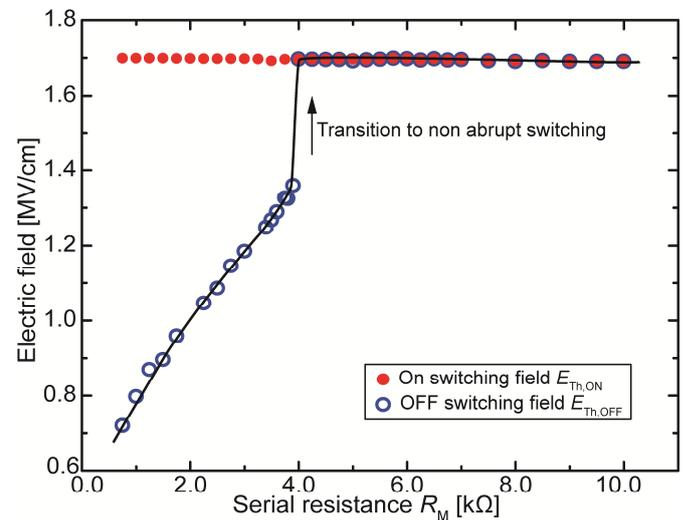
Fig. 4 The switching electric fields are determined by the average electric field in the TS region. The electric field for the turn-on  $E_{Th,ON}$  is determined by the point where the electric field is reduced with increasing applied voltage, which equals the maximum of the averaged electric field. The turn-off electric field  $E_{Th,OFF}$  is determined at the point of increasing electric field after the turn-on.
