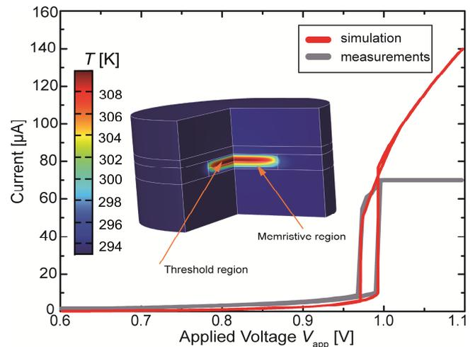
Fig. 1.  $I-V$  characteristics of the FTTR type threshold switching (red) model in comparison with measurement (grey) obtained by an 1T1M ReRAM memory cell. As inset the simulated axial symmetric structure is shown containing the metal electrodes and the insulating area. The filament in the middle is divided into a memristive region and a threshold switching region. The temperature distribution is taken at the onset voltage  $V_{Th,ON}$ .
