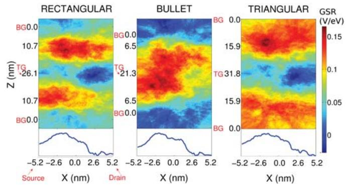
Fig. 4. 2D gate sensitivity profiles for  $V_T$  for the three cross-section shapes (top) and 1D aggregated gate sensitivity along the transport direction (bottom). The top of the gate (TG) and the bottom of the gate (BG) regions are indicated in the figure. The results have been obtained at a low drain bias of 0.05 mV.
