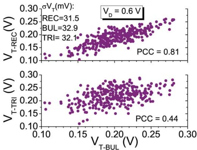
Fig. 5. Scatter plots of  $V_T$  from the rectangular (REC) and triangular (TRI) shapes vs.  $V_T$  from the bullet (BUL) shape due to MGW variations.  $\sigma V_T$  and Pearson correlation coefficient (PCC) are shown for comparison.
