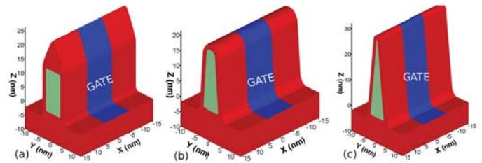
Fig. 1. Schematics of the 10.4 nm gate length (a) rectangular-, (b) bullet- and (c) triangular-shaped channel  $\text{In}_{0.53}\text{Ga}_{0.47}\text{As}$  FinFETs. Dimensions and parameters are summarised in Tables I and II.
