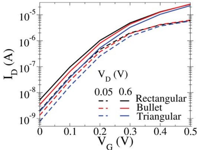
Fig. 2. Sub-threshold region  $I_D$ - $V_G$  curves at both low and high drain biases for three cross-section shapes (rectangular, bullet and triangular) of the 10.4 nm gate length InGaAs FinFET.
