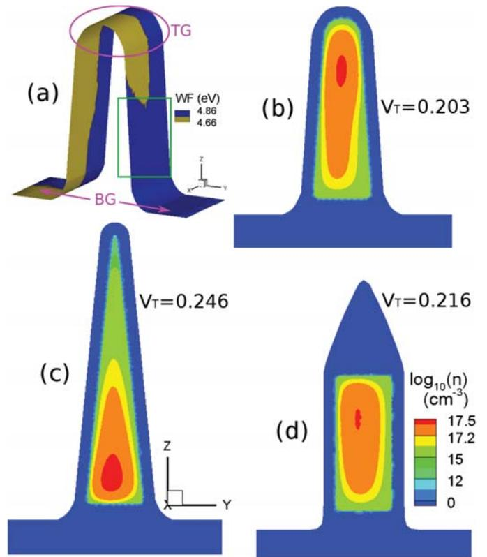
Fig. 3. (a) Example of a MGW profile (with  $GS=7$  nm) applied to the TiN metal gate. Electron density cross-section in the middle of the gate of the FinFET for the same profile with (b) bullet, (c) triangular or (d) rectangular shape at  $V_G=V_T$  and  $V_D=0.6$  V.  $V_T$  values for each shape are also shown.
