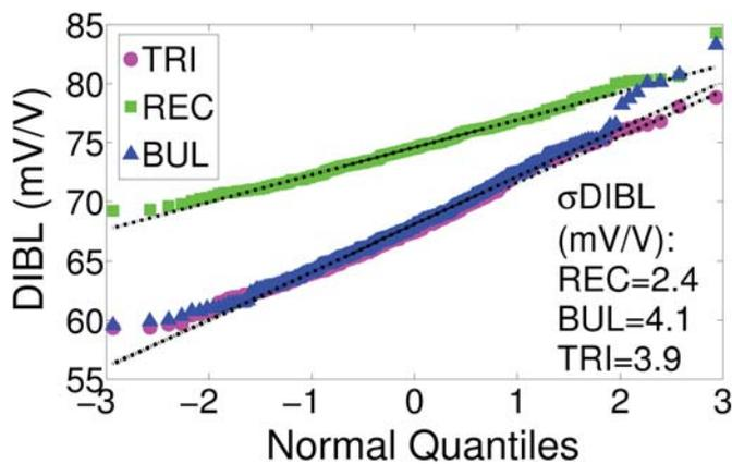
Fig. 6. Q-Q plot for DIBL due to MGW variability for the three cross-sections (REC, BUL, TRI).  $\sigma$ DIBL for the three device shapes is also shown for comparison.
