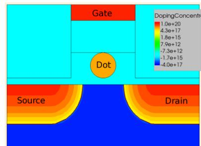
Fig. 1. Scheme of a silicon dot single-electron memory cell with doping distributions in silicon. n-type – positive doping levels in the source/drain doped regions, p-type – negative doping levels in the silicon body. Doping concentration is shown in  $\text{cm}^{-3}$ .
