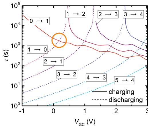
Fig. 7: Charging and discharging time constants for a dot diameter of 6 nm and a tunneling oxide thickness of 3 nm. Each line stands for a certain transition, the respective electron numbers are shown in the figure next to each line. The circle denotes the position, where states  $N_e = 0$  and  $N_e = 1$  have their maximum mutual lifetime.
