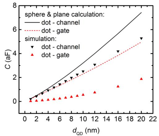
Fig. 3: 3D numerically simulated capacitances between the dot and gate and substrate electrodes in comparison to an analytical description of a conducting sphere and an infinite plane electrode.
