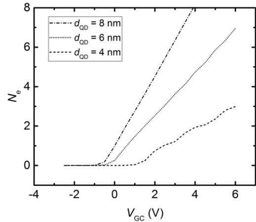
Fig. 5: Equilibrium charge state for different dot sizes dependent on the gate-channel bias voltage. The step-like appearance for low diameters is due to the larger spacing between energy levels for smaller dots.
