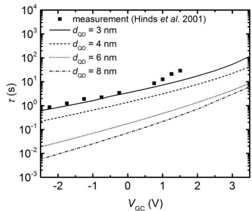
Fig. 6: Calculated electron lifetimes after charging at 6 V in comparison to experimental values by Hinds *et al.* [5].
