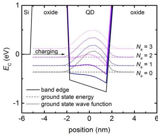
Fig. 4: Conduction band edge and ground state in a 4 nm dot at 6 V bias for different charge states  $N_e$ . The substrate/oxide interface is at -5 nm, the arrow indicates tunneling from the substrate to the dot. Only charge states with energy below the substrate band edge can receive an additional electron.
