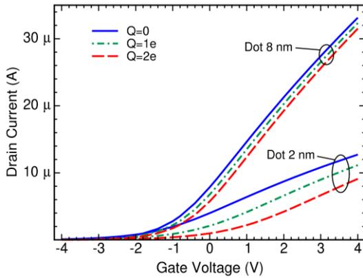
Fig. 2: Impact of the dot-charge state (charge on the dot  $Q=0$ , one electron, and two electrons) on the drain current at a drain voltage of 0.1 V of the MOSFET structure envisaged for the memory-cell-state reading for silicon dot diameters of 2 and 8 nm, respectively.
