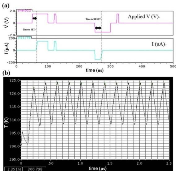
Fig. 6. (a) Pulse voltage, current curve during programming, (b) simulated transient temperature curve in 3D RRAM array.
