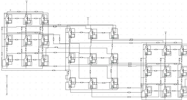
Fig. 5. Circuit diagram of 3D RRAM array.
