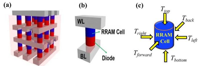
Fig. 1 Schematic diagram of 3D 1D1R crossbar structure (a), and 1D1R storage element (b), and (c) six-direction inputs of temperature.
