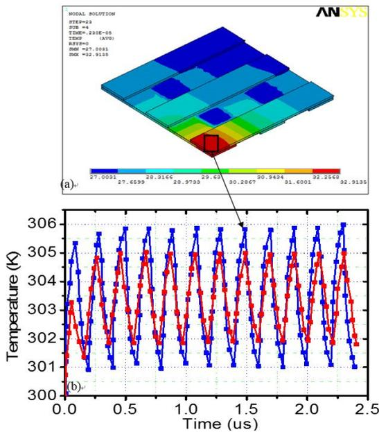
Fig. 9. RRAM  $2 \times 2 \times 2$  array simulation results in ANSYS, here two rows RRAM cells are applied by pulse voltage.
