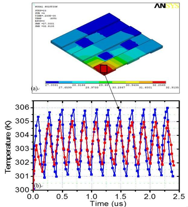
Fig. 8. RRAM 1x1x1 array simulation results in ANSYS, only a single RRAM cell is applied by pulse voltage.
