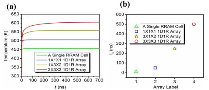
Fig. 3. Highest temperature evolution in the programmed RRAM cell with selected array structures in Fig. 2. (b)  $t_s$  (the time reaching thermal steady state) as a function of array.
