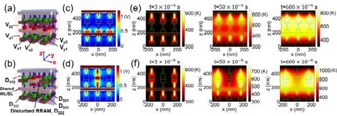
Fig. 4. (a)-(b) Schematic diagram of two selected ‘worst cases’ in thermal crosstalk. (c)-(d) Potential maps in the array structures in (a)-(b). (e)-(f) Temperature maps of the cross-sections (blue planes in (a)-(b)) for two array structures at different time, respectively. Disturbed RRAM device (labeled as D222) locates in the center of the array, which is surrounded by several programmed RRAM cells.
