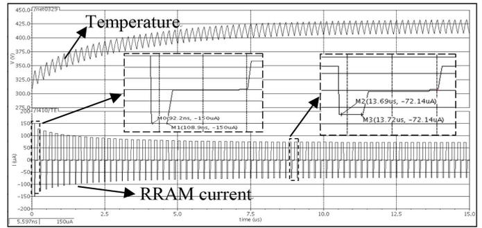
Fig. 7. Simulated temperature and current curves of center RRAM cell operation in 3D RRAM array applied pulse voltages.
