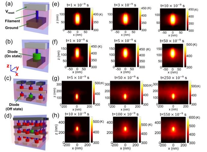
Fig. 2. Schematic diagram of the device structure: (a) an individual RRAM cell, and (b)-(d) ID1R crossbar blocks with 1×1×1, 3×1×2, and 3×3×3 array, respectively. (e)-(f) Temperature evolution maps of the cross-sections (blue planes) in (a)-(d), respectively.
