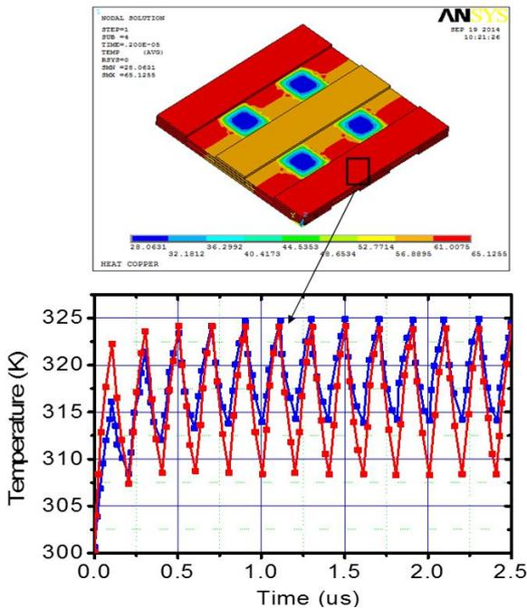
Fig. 10. RRAM  $3 \times 3 \times 3$  array simulation results in ANSYS, here two rows in 3 layers RRAM cells are applied by pulse voltages.
