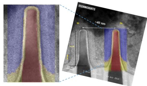
Fig. 1. Fin cross-section generated by GSS structure editor, including the fin, gate oxide and STI, against the TEM image
