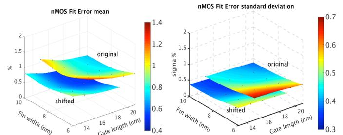
Fig. 12. The fitting errors of statistical compact models with respect to TCAD results.
