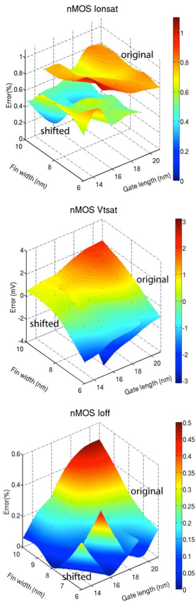
Fig. 10. The extraction errors of compact models with respect to TCAD results over both the shifted DoE and the original DoE, showing excellent accuracy achieved for Figures of Merits.
