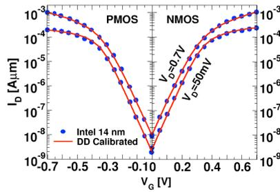
Fig. 3. Device Id-Vg characteristics obtained from calibrated TCAD decks against silicon measurements
