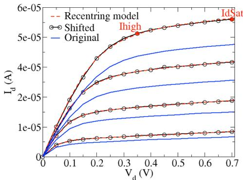
Fig. 8. IdVd characteristics of re-centering model against TCAD results.
