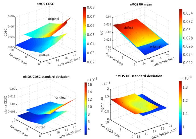
Fig. 11. The mean and standard deviation of some BSIM-CMG parameters extracted from statistical compact modelling for both original and shifted design.
