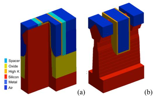
Fig. 2. The 14nm FinFET structure generated by GSS structure editor
