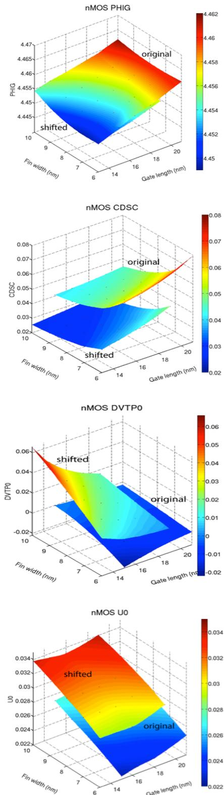
Fig. 9. BSIM-CMG parameter distributions over the shifted DoE space comparing to the original DoE.
