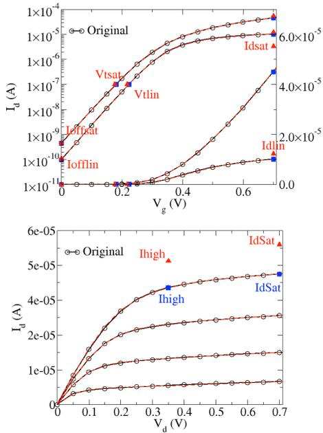
Fig. 7. FoM target used in compact model re-centering study
