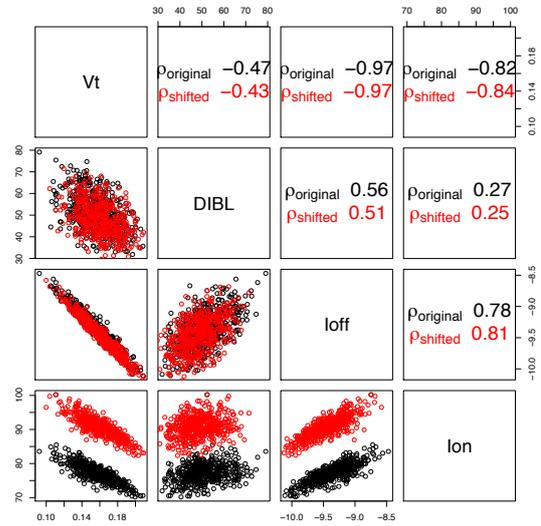
Fig. 5. Statistical TCAD simulations, showing the correlations between Figures of Merits for TT nFinFETs at original and shifted design point, highlighting the good control of subthreshold performance, and much improved drivability in shifted design
