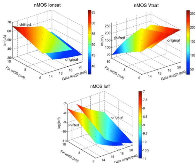
Fig. 4. Figures of Merits for nFinFETs, showing moving from the original DoE to the shifted DoE
