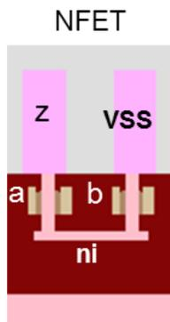
Fig. 13. NFET cross-section of design B
