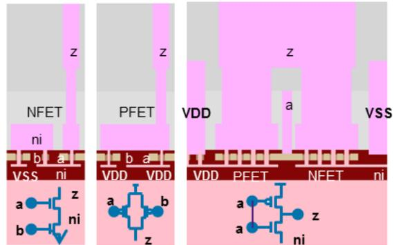
Fig. 8. 2D cross-sections of design A along cell width and cell height directions
