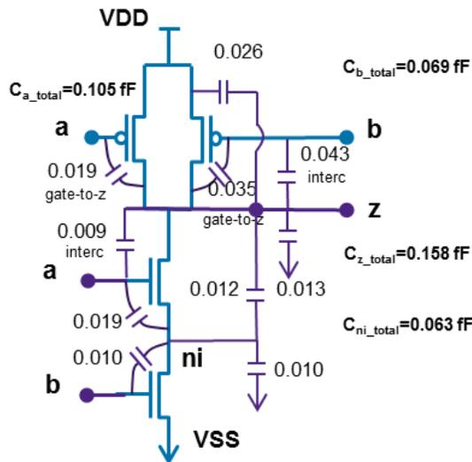
Fig. 10. Parasitic capacitances for design A
