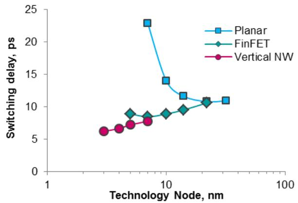
Fig. 4. Benchmarking performance of a 2x inverter built on planar, FinFET, and NW technology with fan-out of 1 and BEOL wire length of 70 metal pitches
