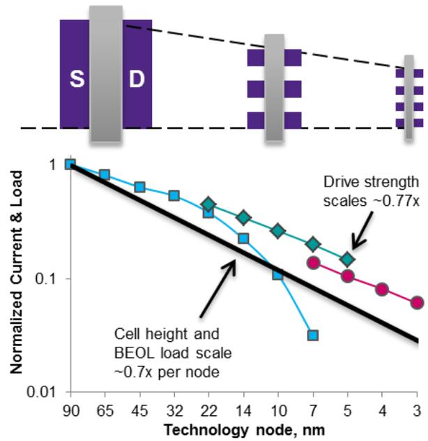
Fig. 2. Transistor strength evolution per layout footprint scaled along with library cell height scaling
