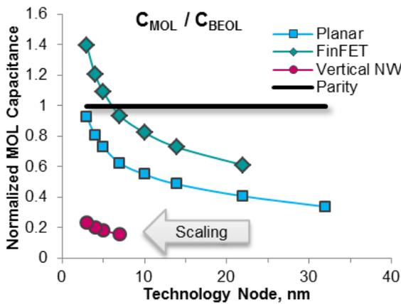
Fig. 3. Evolution of MOL capacitance w.r.t. BEOL capacitance for BEOL wire length of 70 metal pitches
