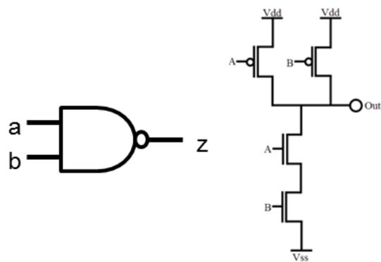
Fig 5. Two-input NAND logic cell
