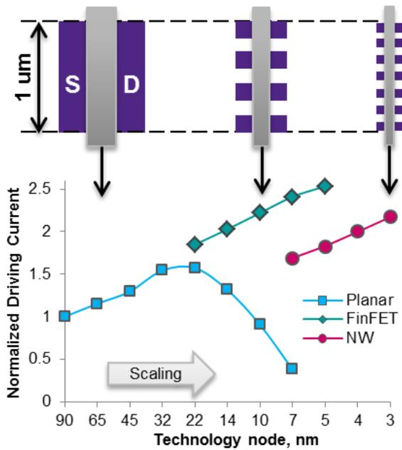
Fig. 1. Transistor strength evolution per 1 μm layout footprint and fixed off-state current and power supply
