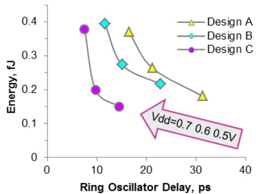
Fig. 14. Benchmarking ring oscillators built on 5nm NW's with different cell design options
