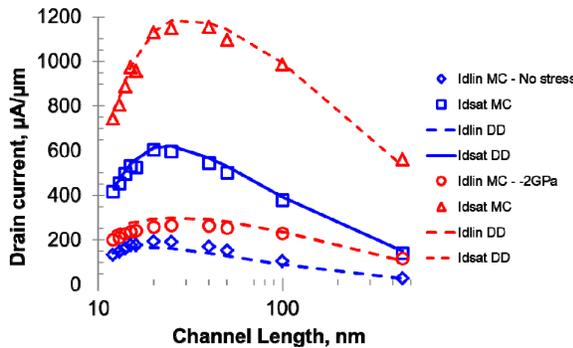
Fig. 9. Monte Carlo simulation vs Drift-Diffusion model with ballistic mobility for 3D P-FinFET ( $L_g=12\text{nm}-450\text{nm}$ , channel stress=0GPa,2GPa)
