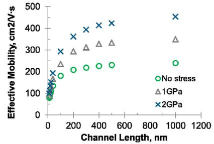
Fig. 5. Effective mobility from Monte Carlo simulation vs. channel length for different channel stresses
