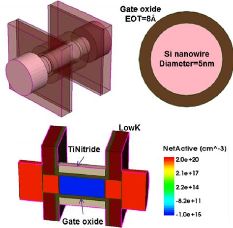
Fig. 10. Gate-all-around (GAA) nanowire geometries and doping (Channel length=11nm. NW channel diameter=5nm. Source/drain diameter=10nm. EOT=8Å. Fin pitch=16nm. Gate pitch=30nm. VDD=0.7V. Undoped channel and source/drain doping of  $2e20\text{cm}^{-3}$ .)
