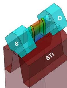
Fig. 2. 3D N-FinFET view (Channel length split from 12nm to 450nm. Fin width=5nm. EOT=8.5Å. Fin pitch=45nm. Gate pitch=60nm. VDD=0.7V. Undoped channel and source/drain doping of  $2e20\text{cm}^{-3}$ .)
