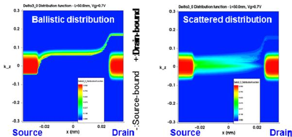
Fig. 13. Distribution functions for nanowire with ballistic transport and with phonon and surface roughness scattering
