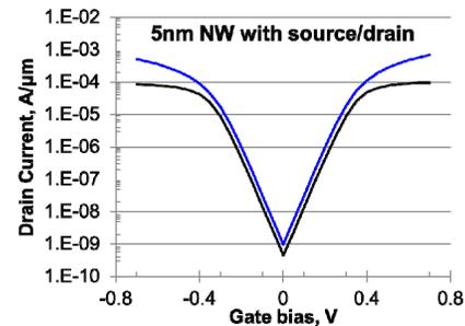
Fig. 12. Nanowire: Extended Drift-Diffusion with the source/drain model
