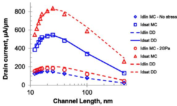
Fig. 8. Monte Carlo simulation vs Drift-Diffusion model with ballistic mobility for 3D N-FinFET ( $L_g=12\text{nm}-450\text{nm}$ , channel stress=0GPa,2GPa)
