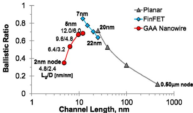
Fig. 14. Evolution of ballistic ratio for planar FETs, FinFETs, and nanowires (Ballistic ratio is for the historic transistor scaling in the industry down to 14nm node and it is projected for the expected transistor scaling down to 2nm node.)
