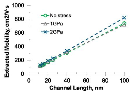
Fig. 7. Ballistic mobility for different stress levels
