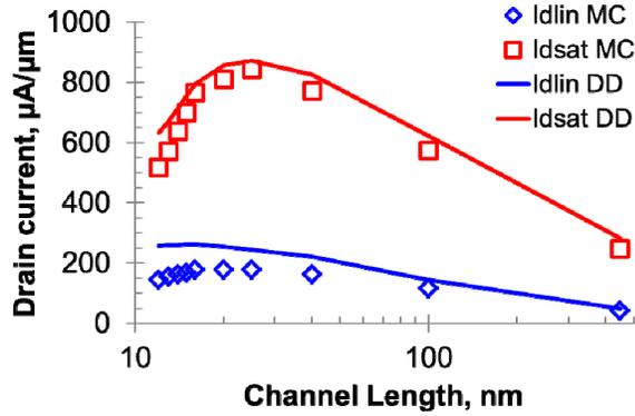
Fig. 3. N-FinFET with 2GPa tensile stress w/o ballistic mobility in Drift-Diffusion (Off-state current=1 nA/µm)
