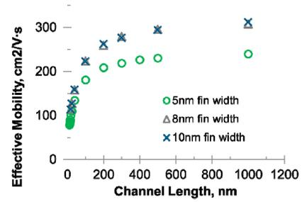
Fig. 4. Effective mobility from Monte Carlo simulation vs. channel length for different fin widths
