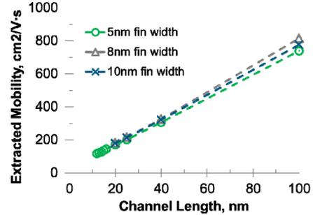
Fig. 6. Ballistic mobility for different fin widths
