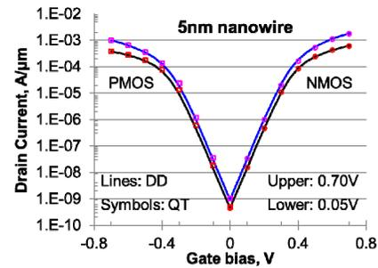
Fig. 11. Nanowire: Quantum Transport & Drift-Diffusion with ballistic mobility
