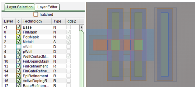
Figure 4. Virtual technology layers are created by logical operations. Combined with the original layer these "helper layers" are used to extrude device segments and boxes for doping profiles.
