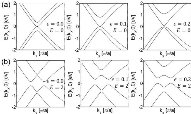
**Fig. 6** Band structure of strained bilayer graphene without (a) and with (b) vertical field [V/nm]. Left, middle and right figures correspond to band structures of bilayer graphene with different strain values.
