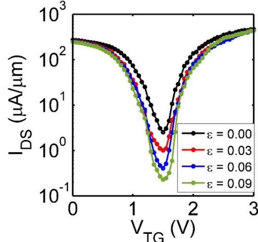
**Fig. 8** IV curves for double gate bilayer graphene devices applied with different vertical strain.
