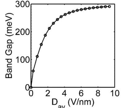
FIG. 2. Dynamic bandgap (DBG) in BLG as a function of the displacement field.
