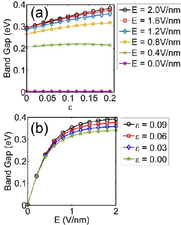
**Fig. 7** (a) Band gap changes with strain applied in different vertical fields [V/nm]. (b) Band gap increases with vertical field. Saturation band gap increases with larger strain.
