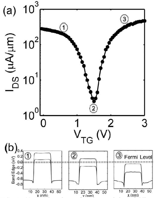
**FIG. 5.** (a): V shaped transfer characteristics of bilayer graphene double gate FET. (b): band edge plot along transport direction for the ON, OFF and ON state.
