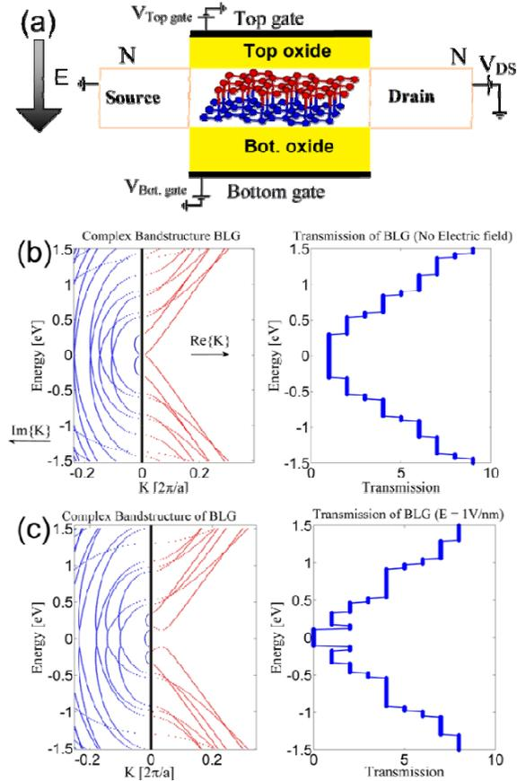
FIG. 3. (a): Bilayer graphene FET device and atomic structure. Bandgap and transmission for a BLG device in a small (b) and large (c) electric field.
