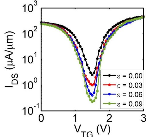
**Fig. 8** IV curves for double gate bilayer graphene devices applied with different vertical strain.
