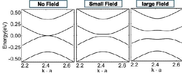
FIG. 1. Bandgap of bilayer graphene changing with a vertical electric field. The bandgap increases with an increasing field up to a saturation point.
