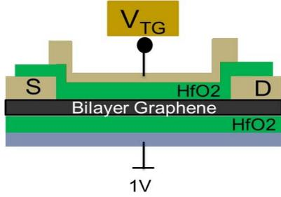
**FIG. 4.** Schematic of the double gated bilayer graphene field effect transistor used in this work.
