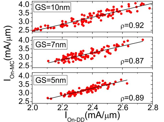
Fig. 3. Scatter plot of the on-current from the MC vs. the DD due to MGW variations for three different grain sizes (GSs). The correlation coefficient ( $\rho$ ) is shown for comparative purposes.
