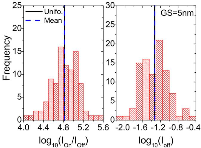
Fig. 6. Distribution of the  $I_{On}/I_{Off}$  ratio and of the off-currents from DD simulations due to MGW variability for a grain size 5 nm. The value for a device with an uniform gate and the mean value of the statistical distribution are included for comparison.
