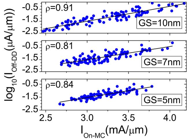
Fig. 5. Scatter plot of the off-current from DD vs. the on-current from MC due to MGW variations for three different grain sizes. The correlation coefficient ( $\rho$ ) is shown for a reference.
