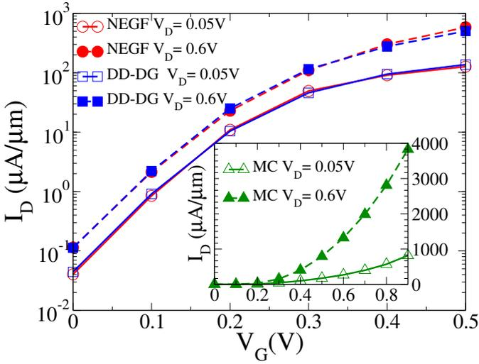
Fig. 1.  $I_D$ - $V_G$  characteristics comparing the 3D DD-DG results against Silvaco's ballistic NEGF simulations [6] on a logarithmic scale at both low (0.05 V) and high (0.6 V) drain biases. The inset shows the Monte Carlo results on a linear scale.
