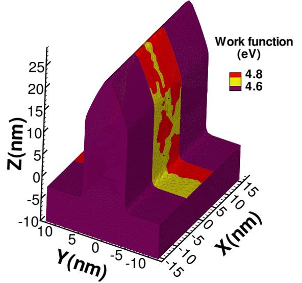
Fig. 2. Example of the TiN metal gate work function variability for a grain size 5 nm. The TiN metal has 2 possible grain orientations with MGWs of 4.8 and 4.6 eV.
