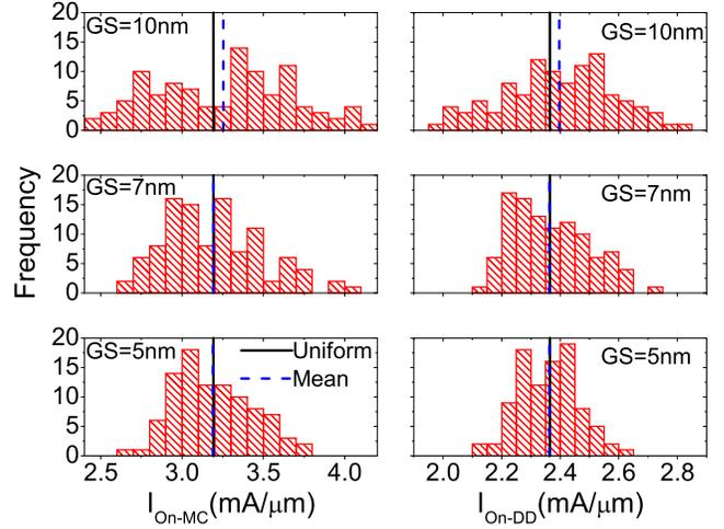
Fig. 4. Distribution of on-currents from MC ( $I_{On-MC}$ ) and DD ( $I_{On-DD}$ ) simulations due to MGW variability for three different grain sizes. The on-current for a device with an uniform gate and the mean value of the statistical distribution are included for comparison.
