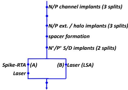
Fig. 2. well, ext./halo and S/D implantation splits and laser annealing sequence studied in this work.
