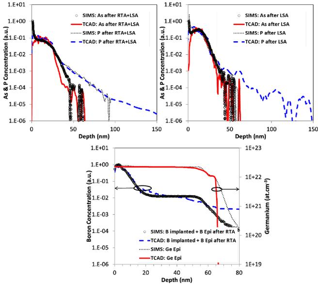
Fig. 4. Comparison of S/D As/Phosphorus co-implantation profiles for RTA+LSA vs LSA for N-type and implanted Boron + Boron Epi profiles after spike-RTA for P-type. Ge content is shown on the right axes. Good agreement is achieved between TCAD and SIMS.
