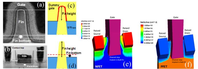
Fig. 3. XTEM images (a) across fin and (b) across gate. x-section acrossfin (c) before dummy gate removal and (d) after dummy gate removal [9]. (e) N and (f) P-type Bulk FinFETs simulated structures.
