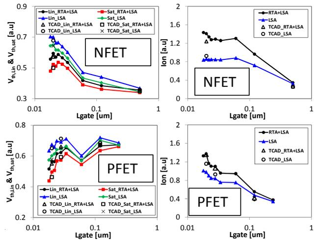
Fig. 6. N-type and P-type bulk FinFET  $V_{th}$  roll-off and  $I_{don}$  characteristic vs.  $L_g$ . TCAD simulations (only long and short devices are reported) well reproduce the measurements especially RTA+LSA vs. LSA. For N-FinFET, Arsenic and Phosphorus co-activation and diffusion is accounted for, and for P-FinFET Boron diffusion account for SiGe effect at S/D region.
