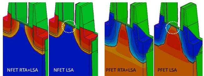
Fig. 7. Net doping variation for RTA+LSA vs. LSA for N and P-type bulk FinFETs. Lower junctions overlap is achieved with LSA only.
