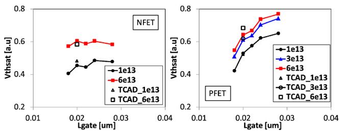
Fig. 5.  $V_{th,sat}$  vs.  $L_g$  with various well dose. And  $V_{th,sat}$  vs. B/As dose of NFET/PFET.  $V_{th}$  modulation is achieved across wide range of  $L_g$  and dose. Good agreement between TCAD (short  $L_g$ ) and experiments.
