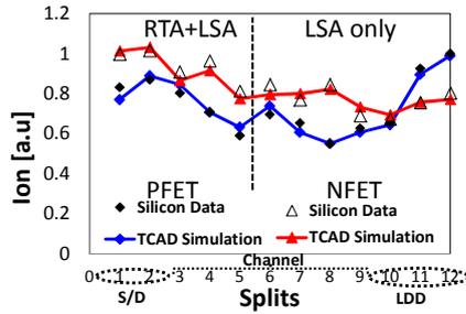
Fig. 8. Ion vs. well, ext./halo and S/D implants splits. The good agreement between TCAD and data demonstrates the accuracy to capture the process variation
