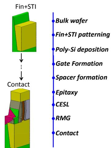
Fig. 1. Bulk FinFET “gate-last” process simulation steps based on process flow.
