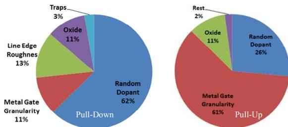
Fig. 10. Pull-Down and Pull-Up mismatch simulation where MGG (metalgategranularity), LER (lineedgeroughness), RDF, OTF (oxidethicknessfluctuation), finthickness variation are included as mismatch sources. Mismatch sources breakdown only possible with the proposed TCAD methodology
