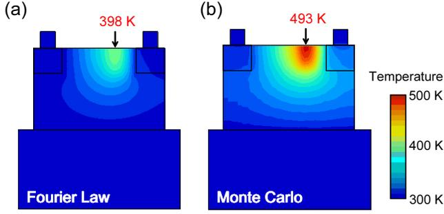
Fig. 3. Steady-state temperature distribution on the vertical cross-section indicated in Fig. 1. The simulation results obtained from (a) the heat conduction equation based on Fourier’s law and (b) the present MC method are compared.
