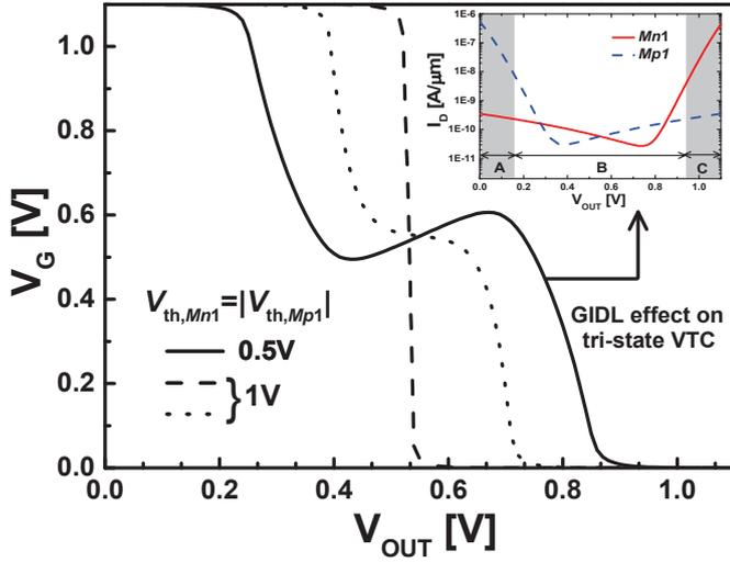
Fig. 2. Voltage transfer curve (VTC) at  $V_{th,Mn1}=|V_{th,Mp1}|=0.5V$  and  $1V$ . GIDL effect makes inclined tri-state VTC with inserted  $I-V$  characteristics of  $Mn1$  and  $Mp1$ .
