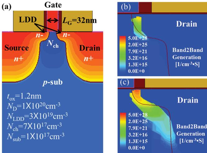
Fig. 3. (a)  $nMOS$  schematic and (b) band-to-band generation view by using 32-nm CMOS technology structure. (c) Band-to-band generation with our enhanced condition
