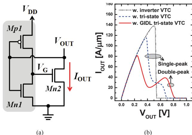
Fig. 1. (a) Proposed NDR circuit scheme and (b) its I-V curve according to various voltage transfer curve (VTC). Inverter VTC and tri-state VTC have single peak NDR characteristics and tri-state VTC with GIDL effect has double peak NDR characteristics.
