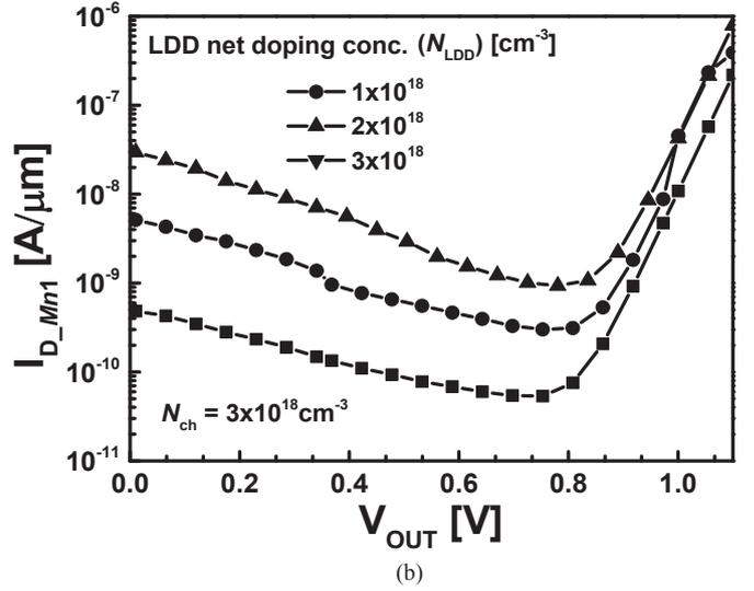
Fig. 4.  $I-V$  characteristic of  $Mn1$  according to (a) various channel doping concentration ( $N_{ch}$ ) and (b) net doping concentration of lightly doped drain ( $N_{LDD}$ )
