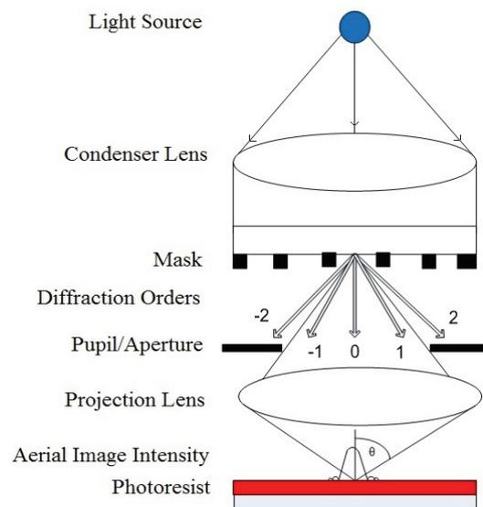
Fig. 1. The block diagram of a projection lithography system
