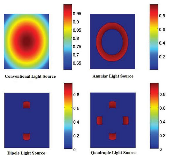
Fig. 2. Four different type of light sources generally used in advanced lithography systems
