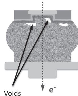
Fig. 2. EM failure is caused by voids which are formed between Ni under bump metalization (UBM) and Sn solder bump.
