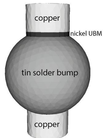
Fig. 5. Structure of the solder bump used for the study. On the top of the Sn bump a Ni UBM is placed.
