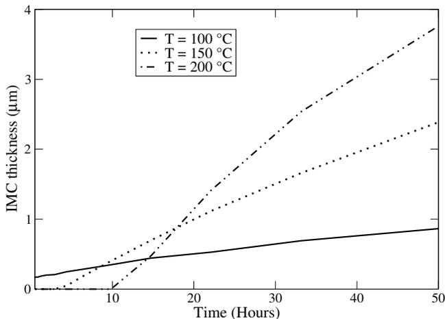
Fig. 8. Growth of IMC thickness in time. Fast migration of Cu and Ni at 150°C and 200°C prevents IMC emergence until 10h of EM stressing.
