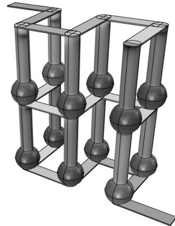
Fig. 4. Multilevel interconnect for 3D integration. Wafers are removed from the picture. Lighter color represents areas with higher current density.
