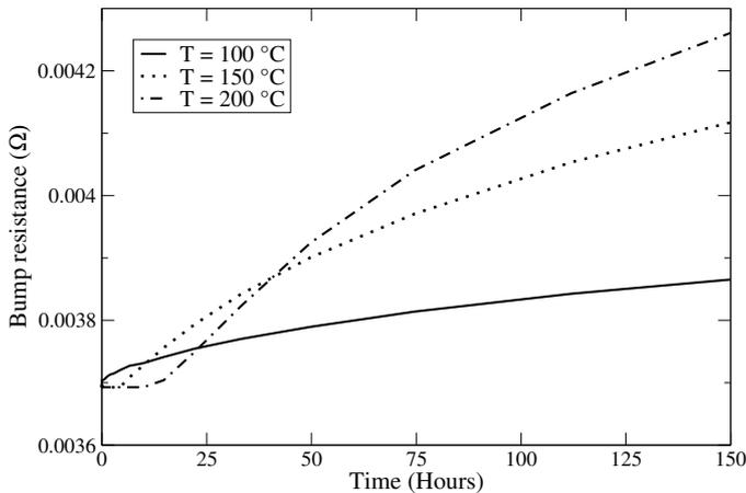
Fig. 7. Initial phase of solder bump resistance growth for three different temperatures.
