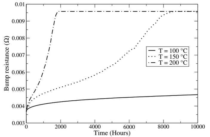
Fig. 9. Late phase of the resistance growth. Resistance of solder bump increases until the whole Sn is converted into IMC.
