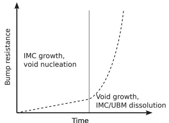
Fig. 3. Resistance change due to IMC growth and voiding with two different slopes.
