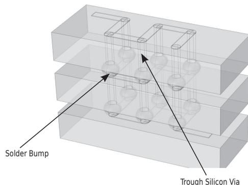
Fig. 1. Schematic representation of wafer stacking by using TSVs and solder bumps.
