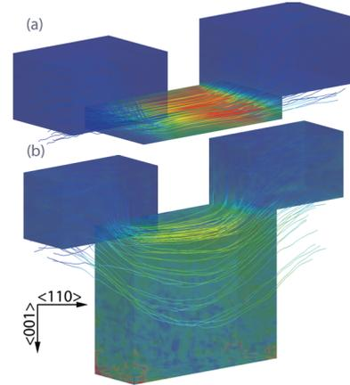
Fig. 15. Velocity vector stream tracer for holes in the p-type (a) IFQW and (b) Tri-gate MOSFETs at  $V_G=0.6V$ .
