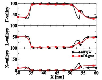
Fig. 14. InGaAs valley occupation through the channel of the n-type IFQW and Tri-gate MOSFETs at  $V_G=0.6V$ .
