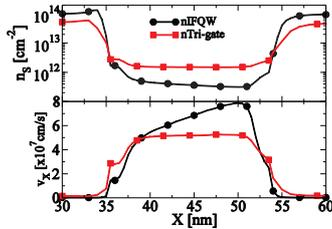
Fig. 11. Sheet electron density and electron velocity through the channel of the n-type IFQW and Tri-gate MOSFETs at  $V_G=0.6V$ .
