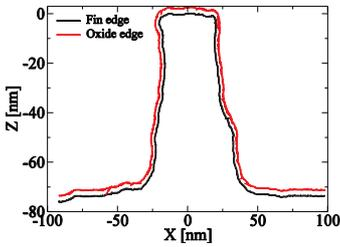
Fig. 4. Extracted fin profile for a  $W_{fin}=45nm$  tri-gate FET from Radosavljevic *et al.* 2011 [10].
