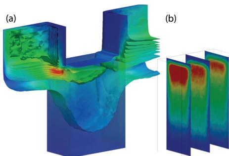
Fig. 18. (a) Electron equi-concentration contours coloured by current density through the fin channel of raised source/drain tri-gate MOSFET. (b) Current density slices through the fin channel of the raised source/drain tri-gate MOSFET.
