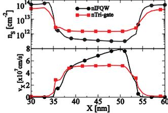
Fig. 11. Sheet electron density and electron velocity through the channel of the n-type IFQW and Tri-gate MOSFETs at  $V_G=0.6V$ .
