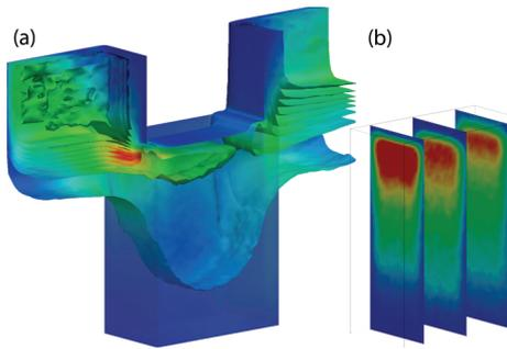
Fig. 18. (a) Electron equi-concentration contours coloured by current density through the fin channel of raised source/drain tri-gate MOSFET. (b) Current density slices through the fin channel of the raised source/drain tri-gate MOSFET.
