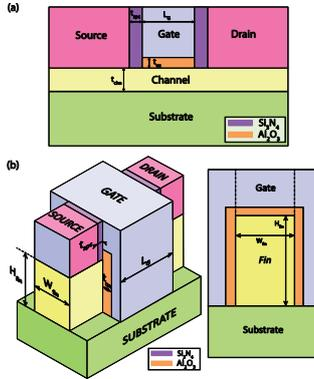
Fig. 3. Structure of (a) the Implant-Free Quantum-Well and (b) the Implant-Free Tri-gate MOSFET architectures.
