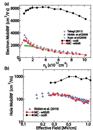
Fig. 2. Universal mobility characteristic of (a) InGaAs and (b) Ge from Monte Carlo simulation against experimental data.
