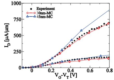
Fig. 6. Monte Carlo results of drive current against published data from Radosavljevic *et al.* [10].
