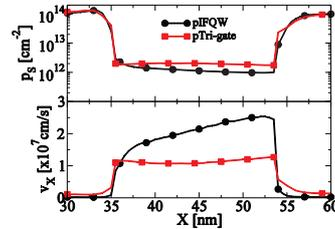
Fig. 12. Sheet hole density and hole velocity through the channel of the p-type IFQW and Tri-gate MOSFETs at  $V_G=0.6V$ .
