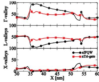
Fig. 13. InGaAs valley occupation through the channel of the n-type IFQW and Tri-gate MOSFETs at  $V_G=1V$ .
