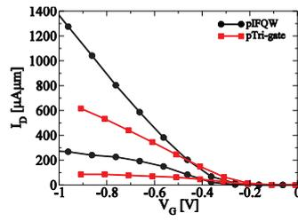
Fig. 8.  $I_D$ - $V_G$  characteristic of the p-type IFQW and Tri-gate MOSFETs for a fixed  $I_{OFF}=0.1 \mu A/\mu m$ .
