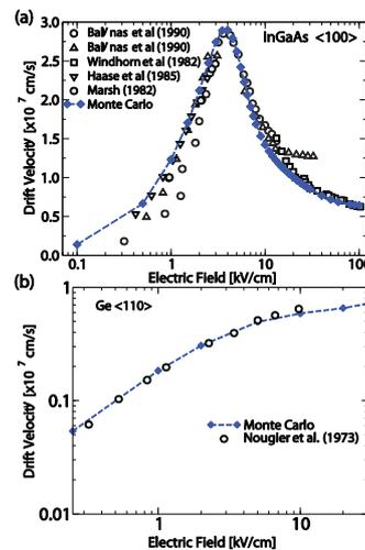
Fig. 1. Velocity-field characteristic of (a) InGaAs and (b) Ge from Monte Carlo simulation against experimental data.
