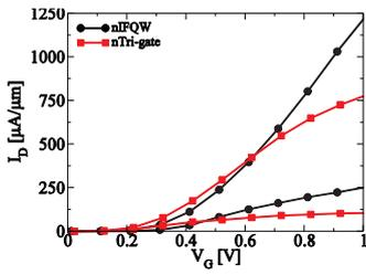
Fig. 7.  $I_D$ - $V_G$  characteristic of the n-type IFQW and Tri-gate MOSFETs for a fixed  $I_{OFF}=0.1 \mu A/\mu m$ .
