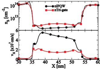
Fig. 9. Sheet electron density and electron velocity through the channel of the n-type IFQW and Tri-gate MOSFETs at  $V_G=1V$ .
