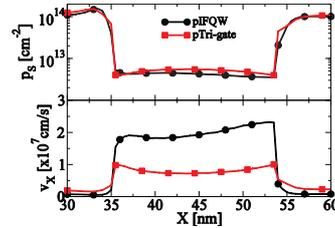
Fig. 10. Sheet hole density and hole velocity through the channel of the p-type IFQW and Tri-gate MOSFETs at  $V_G=0.9V$ .
