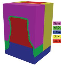
Fig. 5. Device structure with extracted fin profile  $W_{fin}=45nm$  as used in the GARAND simulator.
