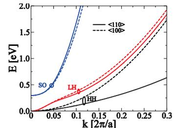
Fig. 17. E-k relation of the warped Ge bandstructure for two different transport directions.
