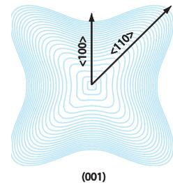
Fig. 16. Equi-energy contours on the (001) plane in k-space of the Ge bandstructure for Heavy Holes (HH).
