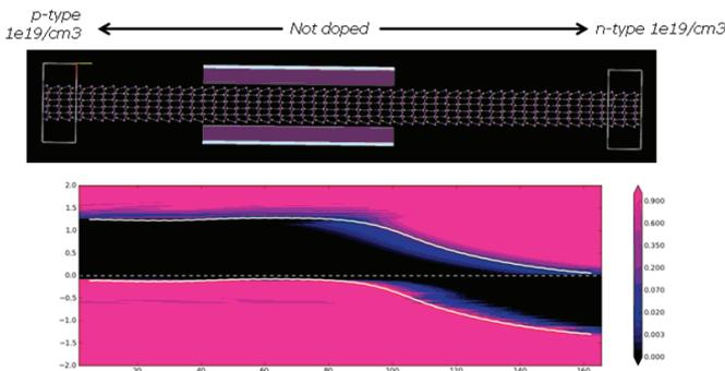
Fig. 4. Geometry of the 2D InAs p-i-n junction of width 13 Å and length 166 Å. Periodic boundary conditions are used in the direction perpendicular to the viewplane. An electrostatic double gate is placed in the center of the device, and a 6 Å thick dielectric is inserted between the gate and the device. The lower figure shows the DFT LDOS of the device at zero applied bias and with the gate potential grounded to the left electrode. The dashed line shows the Fermi level of the system.
