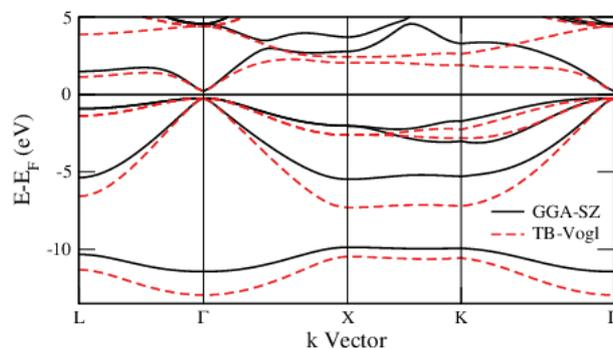
Fig. 1. Bandstructure of InAs obtained with the special DFT-GGA basis set and the Vogl TB model. Note the similar bandgap obtained with the two methods. The Fermi level is positioned in the middle of the band gap, and defines the energy zero level.
