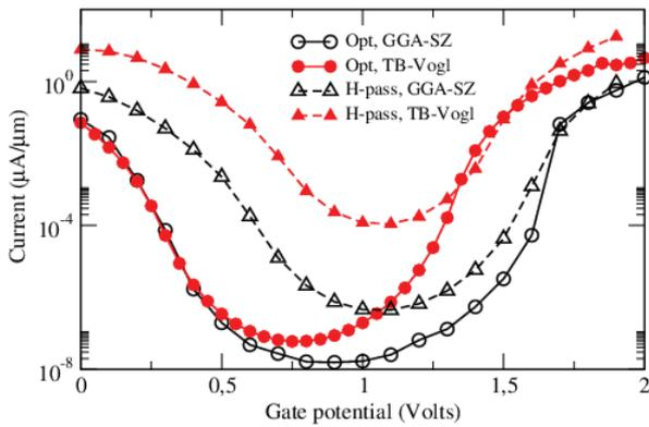
Fig. 6. Current-gate characteristics for an applied bias of  $-0.5$  V. Zero gate potential corresponds to the gate grounded to the left electrode. The ground of the right electrode is at 1.58, 1.68, 1.78, 1.53 V for the different models, respectively.
