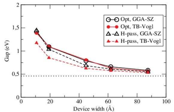
Fig. 3. Bandgap as function of the width of the InAs device system.
