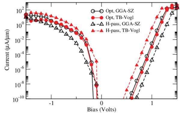
Fig. 5. Current-voltage characteristics for the p-i-n junction, with the gate grounded to the left electrode (zero gate). A positive bias corresponds to forward bias of the p-n junction. The current is calculated for different surface passivation models and with both the DFT and the TB method.
