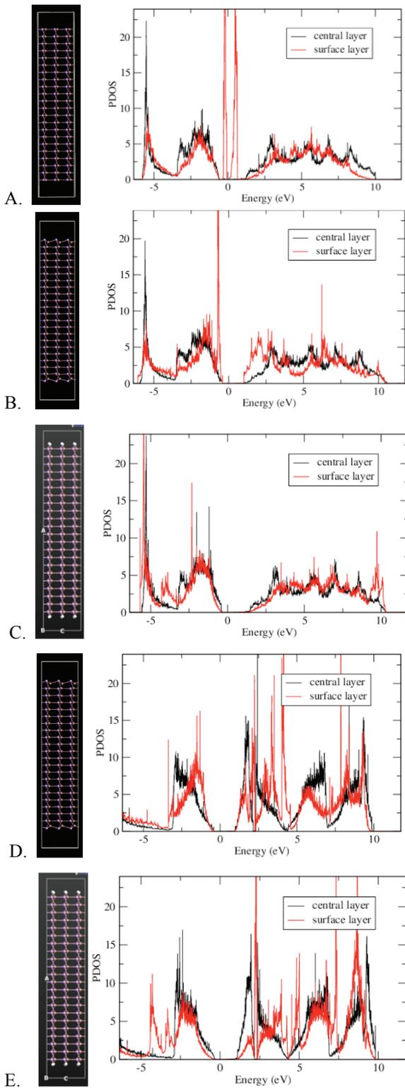
Fig. 2. Projected density of states (PDOS) for the surface and bulk layer of a 46 Å wide InAs 2D system with different surface passivation, and using different methods. A) Bulk surface, DFT, no passivation; B) Relaxed surface, DFT, no passivation; C) H-passivated surface, DFT; D) Relaxed surface, TB, E) H-passivated surface, TB.
