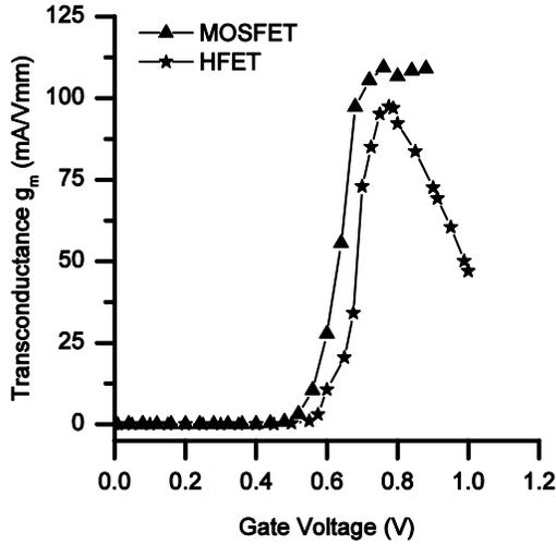
Figure 5: Simulated transconductance ( $g_m$ ) for the MOSFET and HFET with 50um gate lengths.
