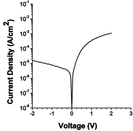
Figure 3: Current characteristics used to calibrate the simulation models and interface quality of the MOS structure.
