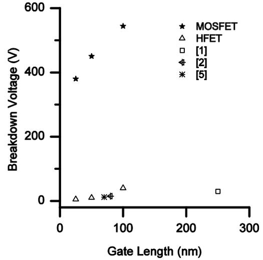
Figure 6: The breakdown voltage versus gate length of the simulated MOSFET and HFET devices compared to current fabricated HFETs.
