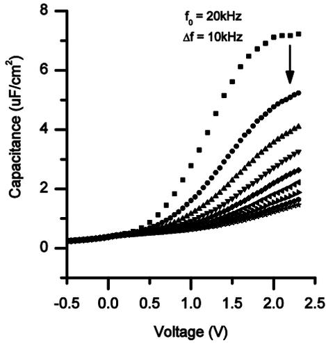
Figure 2: Capacitance measurements used to calibrate the simulation models.
