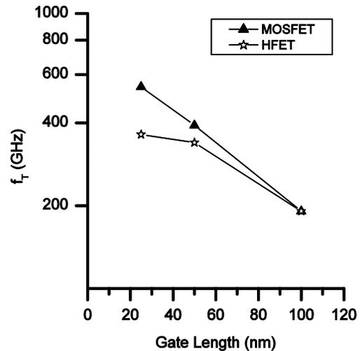
Figure 7: Unity gain frequency comparison for the optimized MOSFET and HFET
