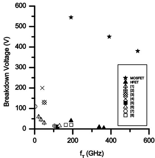
Figure 8: Breakdown frequency compared to unity gain frequency for current technology and the simulated devices.
