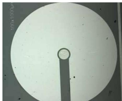
Figure 1: Examine of the planar GaN MOSCAP structure that was used to calibrate the simulation models.
