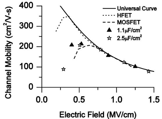
Figure 4: Simulation mobility calibrated to the extracted effective channel mobility of the fabricated test devices. The results follow the universal effective channel mobility for GaN [10].
