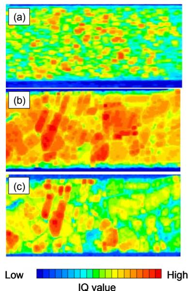
Figure 5. Change of the crystallinity of thin film interconnection: (a) without annealing, (b) annealed at 400°C and (c) three month after annealing
