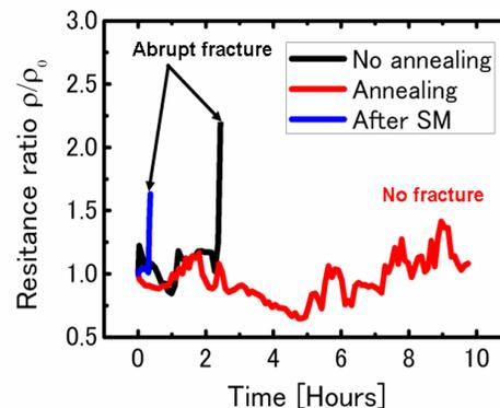
Figure 2. Examples changes of resistance of the thin film interconnections
