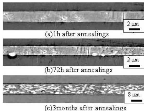
Figure 4. Change of the surface morphology of the annealed electroplated copper thin film interconnection caused by stress-induced migration
