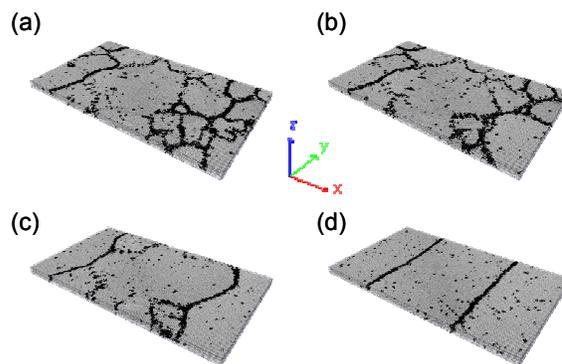
Figure 6. Simulation models of copper thin films, (a) without annealing, (b) annealed at 673 K, (c) annealed at 873 K and (d) annealed at 1073 K. Black color indicates the region of grain boundaries.
