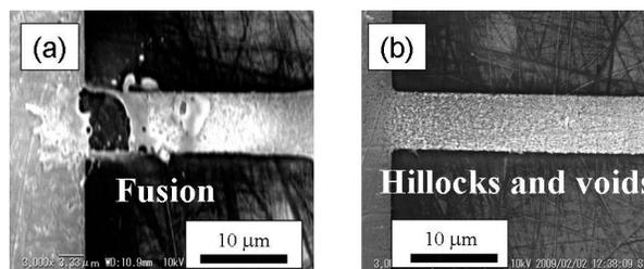
Figure 3. SEM photographs of the surface of the film after electro-migration test; (a) As-electroplated. (b) Annealed at 400°C
