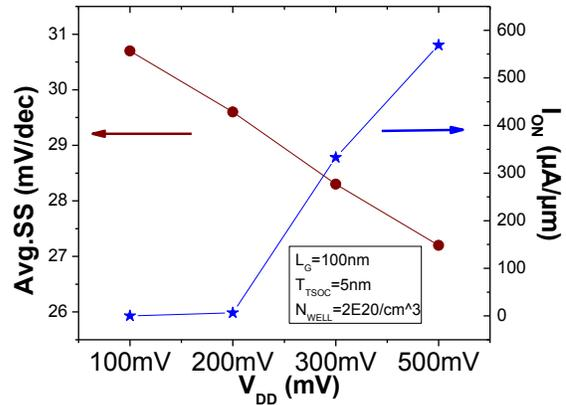
Figure 7. Summary of  $I_{ON}$  and average SS for various  $V_{DD}$ . Average SS is calculated from  $I_{DS}$  of  $1 pA/\mu m$  to  $1 \mu A/\mu m$ . EOT=3nm
