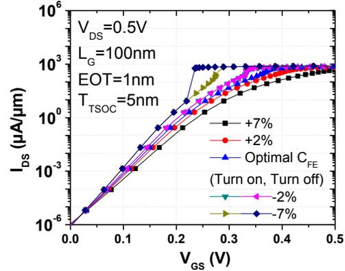
Figure 3.  $I_D$ - $V_G$  for different  $C_{\text{FE}}$  values. +% refers to  $|C_{\text{FE}}|$  larger than the optimal value and no hysteresis in the I-V curve. Optimal  $C_{\text{FE}}$  refers to minimum  $C_{\text{FE}}$  without hysteresis. -% refers to  $|C_{\text{FE}}|$  smaller than the optimal value and hysteresis exists. IV curves shown are  $V_t$  adjusted with  $I_{\text{OFF}}=1\text{E}-6$  at  $V_G=0$ .
