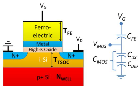
Figure 1 (a) Schematic cross-section views of a NCFET. (b) Simplified capacitance representation of a NCFET.
