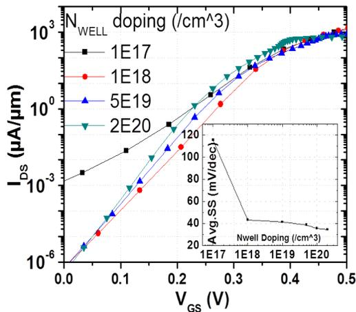
Figure 5. Effects of  $N_{WELL}$  (no hysteresis  $I_D$ - $V_G$ ). The inset shows the average SS for different  $N_{WELL}$  doping.  $V_{DS}=0.5V$ ,  $L_G=100nm$ ,  $T_{TSOC}=5nm$ . IV curves shown are  $V_t$  adjusted with  $I_{OFF}=1E-6$  at  $V_G=0$ . (except  $N_{WELL}=1E17/cm^3$ )
