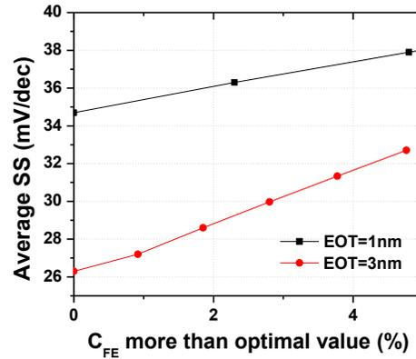
Figure 4. Effects of too large  $C_{\text{FE}}$  on the average SS. When  $|C_{\text{FE}}|$  exceeds the optimal value, the SS degrades.  $V_{\text{DS}}=0.5\text{V}$ ,  $T_{\text{TSOC}}=5\text{nm}$ ,  $L_G=100\text{nm}$ ,  $N_{\text{WELL}}=2\text{E}20/\text{cm}^3$ . Average SS is calculated from  $I_{\text{DS}}$  of 1 pA/ $\mu\text{m}$  to 1  $\mu\text{A}/\mu\text{m}$ .
