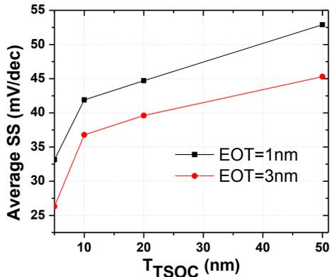
Fig. 6. Effects of  $T_{TSOC}$  and EOT on SS.  $V_{DS}=0.5V$ ,  $L_G=100nm$ ,  $N_{WELL}=2E20/cm^3$ . Average SS is calculated from  $I_{DS}$  of  $1 pA/\mu m$  to  $1 \mu A/\mu m$ .
