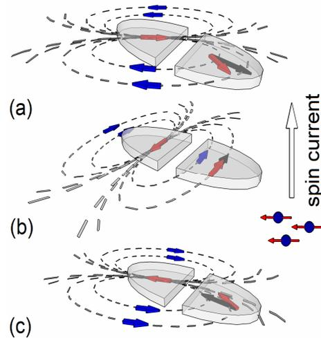
Figure 10. Schematic illustration of the state with self-stabilization direction of the stray magnetic field (a), opposite magnetization state (b), and self-acceleration switching state (c) in an MTJ with a composite free layer.
