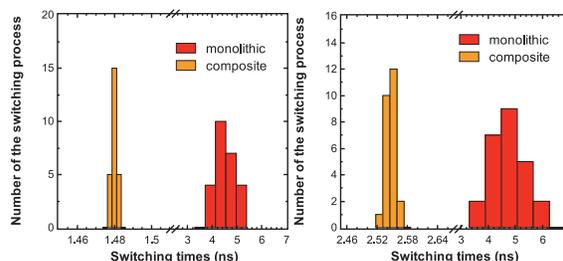
Figure 2. Distributions of the switching times for an MTJ of  $75 \times 25 \text{ nm}^2$  (left) and  $155 \times 60 \text{ nm}^2$  (right) cross-section with monolithic and composite free layer.
