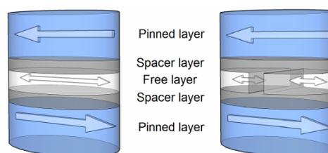
Figure 1. Schematic illustration of penta-layer MTJs with monolithic (left) and composite free layer (right).
