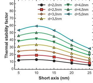
Figure 5. Thermal stability factor for MTJs with monolithic (top) and composite (bottom) free layer as function of the short axis. The long axis is fixed at  $52.5 \text{ nm}$  and the thickness of the fixed layers are  $5 \text{ nm}$ .
