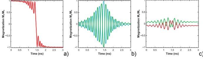
Figure 3. Magnetization components as a function of time for an MTJ element of  $75 \times 25 \text{ nm}^2$  with a composite free layer. The magnetization of the left and right half is shown separately.
