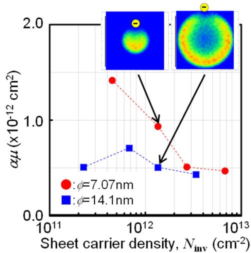
Fig. 6. Relation between the mobility fluctuation term ( $\alpha\mu$ ) and the sheet carrier density. The insets show carrier distributions for each NW.
