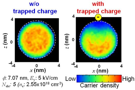
Fig. 4. Carrier distribution at the cross section of the channel without and with a single trapped charge.
