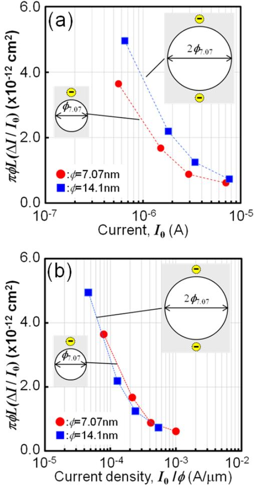
Fig. 7.  $I/I_0$  normalized by surface channel area as a function of (a) current and (b) current density per unit width.  $I_0$  denotes the mean current in case without a trapped charge.
