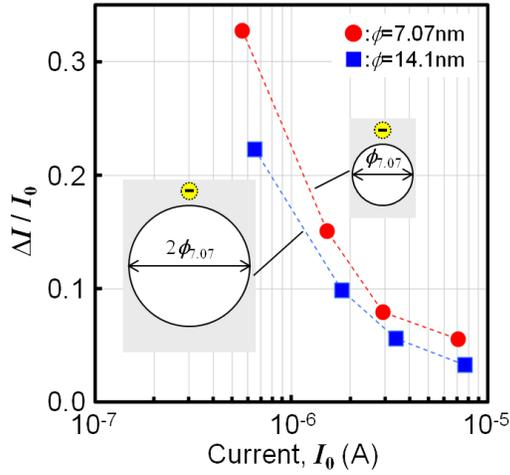
Fig. 5. Relation between the relative amplitude of current reduction and the current.  $I_0$  denotes the mean current in case without a trapped charge.
