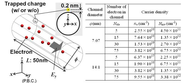
Fig. 2. Simulated gate-all-around channel model and simulation conditions. 1D periodic boundary condition is imposed along the channel.
