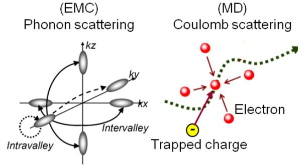
Fig. 1. Scattering processes considered in the EMC/MD method: (1) phonon scattering based on EMC algorithm, and (2) Coulomb scattering among the point charges based on MD algorithm.
