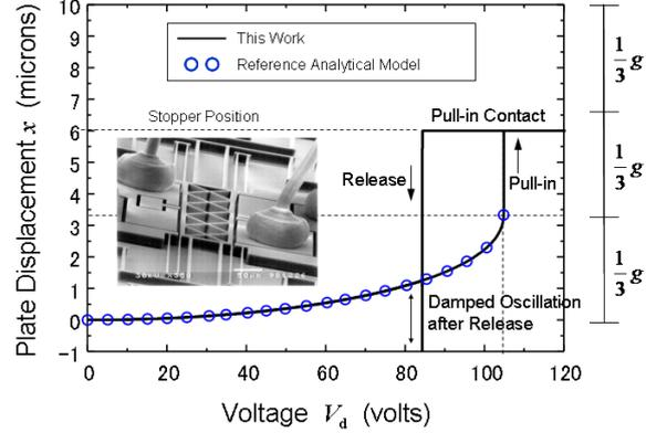
Figure 8. Simulation results of electrostatic parallel plate actuator
