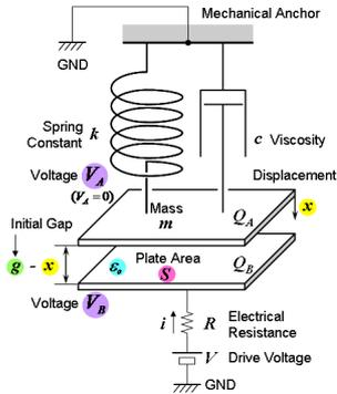
Figure 2. Analytical model for electrostatic parallel plate actuator
