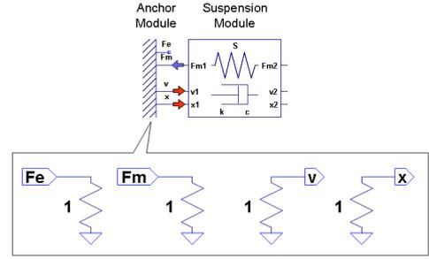
Figure 7. Equivalent circuit model for mechanical anchor
