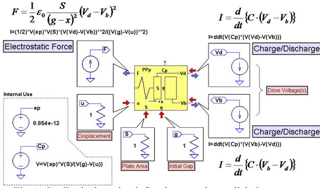
Figure 5. Equivalent circuit for electrostatic parallel plate actuator
