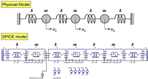
Figure 9. Simulation model for three-body coupled oscillators
