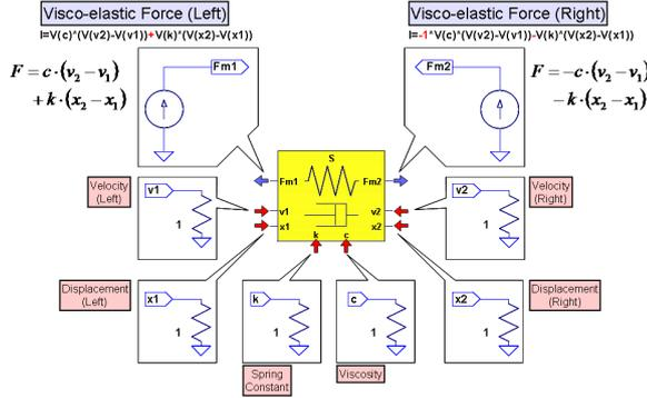
Figure 6. Equivalent circuit model for visco-elastic suspension
