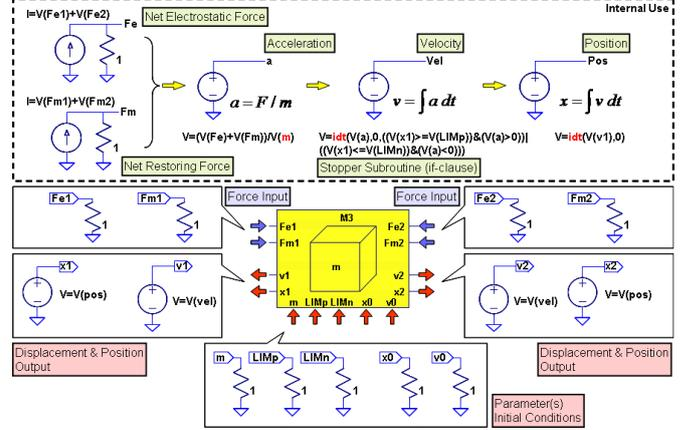
Figure 4. Kernel of the equation-of-motion solver unit
