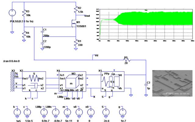
Figure 11. Multi-physics simulation example (silicon resonator)
