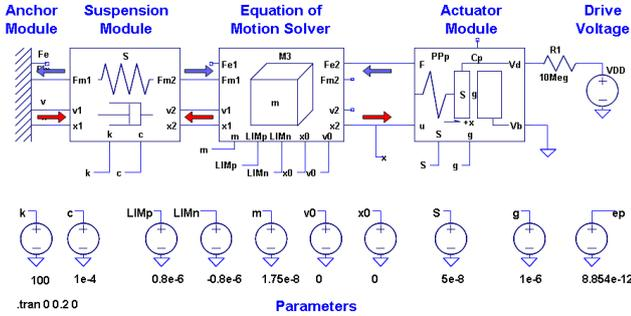
Figure 3. Spice-based MEMS simulation block diagram
