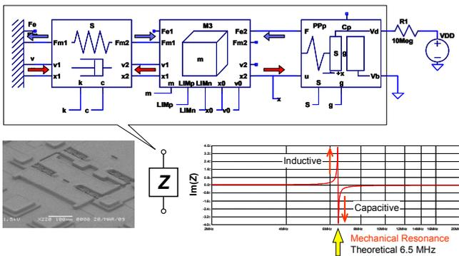
Figure 10. Electrical impedance simulation of electrostatic actuator
