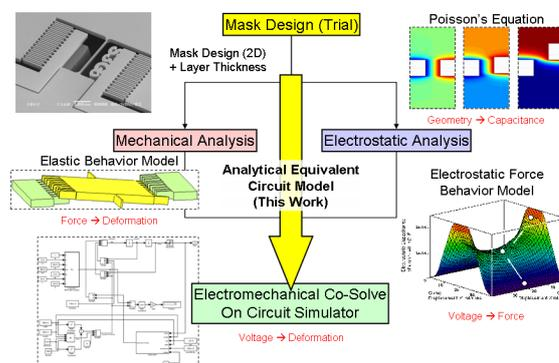
Figure 1. MEMS simulation flow
