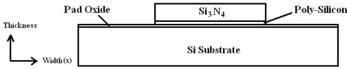
Fig. 1. Schematic structure of the test sample [8]. Width of the nitride/poly-Si is 9.4\mu\text{m} .
