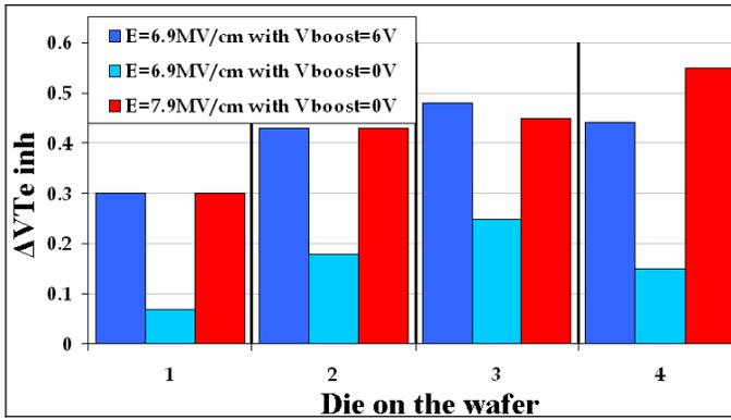
Figure 2. Threshold voltage shift of the erased state after 100,000 cycles
