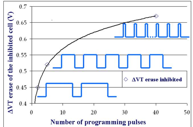
Figure 5. Logarithmic variation of the erased threshold voltage of the inhibited cell after 100,000 cycles as a function of the number of pulses used to reach the same programmed level
