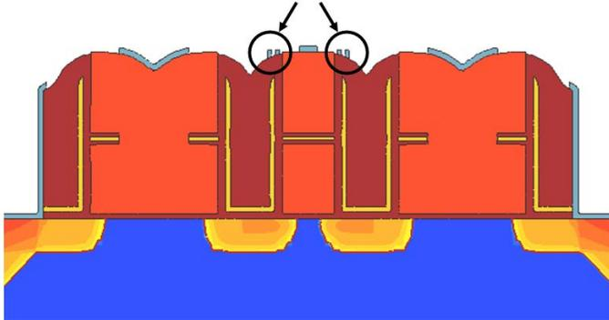
Figure 3. 2D TCAD Process structure, emulating 3D behavior thanks to parasitic capacitance consideration
