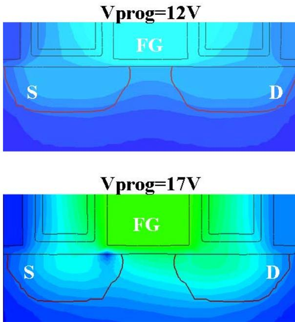
Figure 6. Electrical potential in the transient phase of channel boosting
