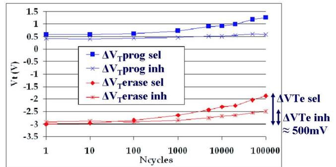
Figure 1. Programmed & Erased  $V_T$  as a function of Write/Erase cycles
