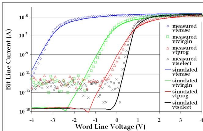
Figure 4. Calibration with  $I_{BL}$  vs.  $V_{WL}$  measurements on erased, virgin, programmed cells and on select transistors.
