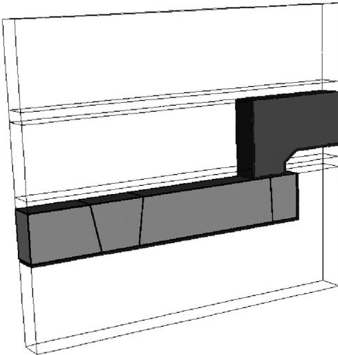
Fig. 2. Dual-damascene structure used for simulation.
