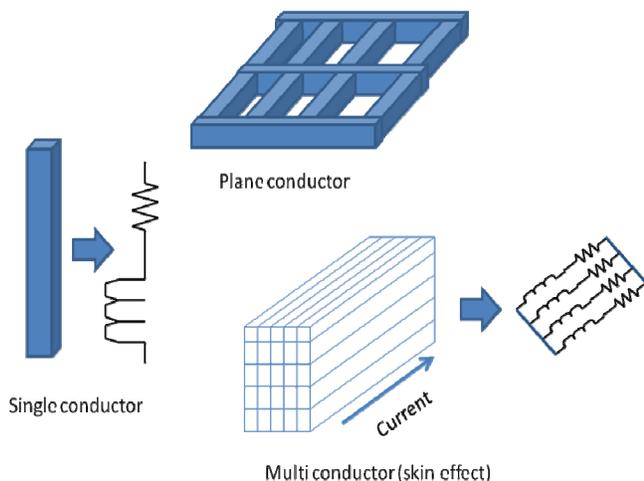
**Figure 7. Representation of conductors for inductance extraction.**
