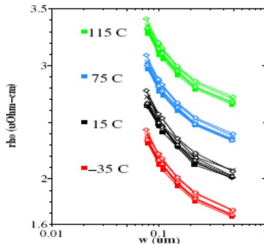
Figure 6. Resistivity of Cu lines as a function of width and temperature. Fig from [5].
