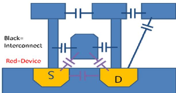
Figure 5. Cross section showing device and interconnect capacitances.
