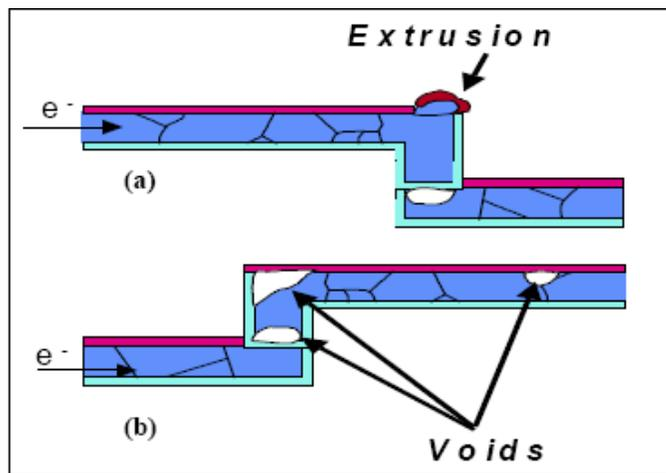
**Figure 9. Voids and Extrusions. Fig from [9].**
