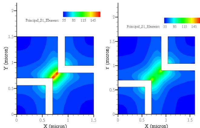
**Figure 8, Stress in low-k dielectric due to CTE mismatch. Fig from 11.**
