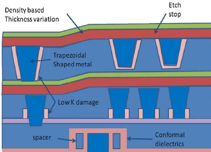
**Figure 1. Technology cross-section showing dielectric.**
